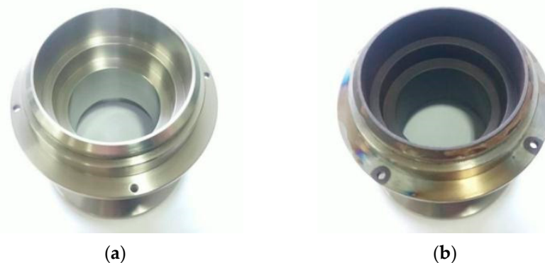
Figure 7. Photographs of the infrared imaging opto-mechanical system: (a) without ceramic coating; (b) with ceramic coating.
