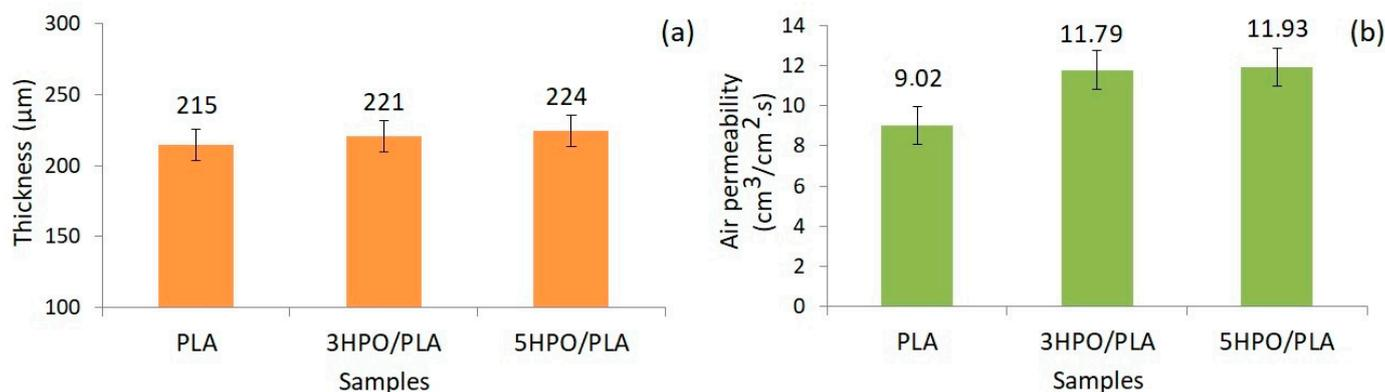
**Figure 4.** The thickness (a) and, air permeability (b) test results of PLA and HPO/PLA electrospun nonwoven fabrics.
