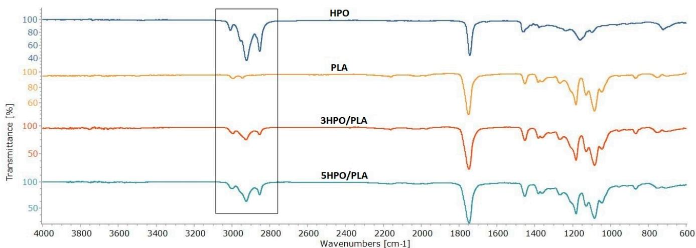
**Figure 2.** ATR-FTIR spectra of the HPO, the PLA, and the HPO/PLA electrospun nonwoven fabrics.
