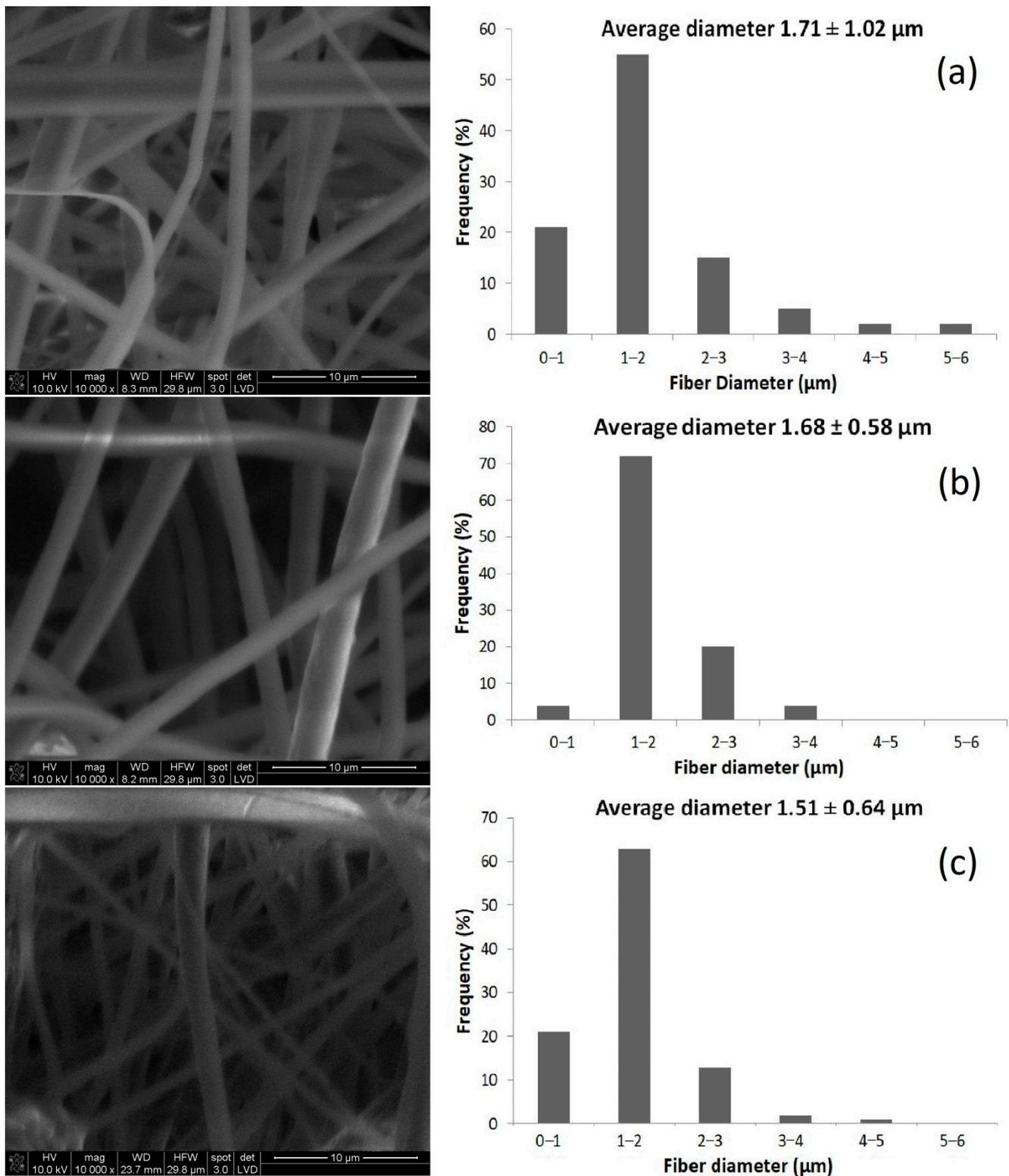
**Figure 1.** SEM images and fiber diameter distributions of the electrospun nonwoven fabrics obtained from (a) PLA, (b) 3HPO/PLA and (c) 5HPO/PLA ( $\times 10,000$ ) (average  $\pm$  standard deviation).
