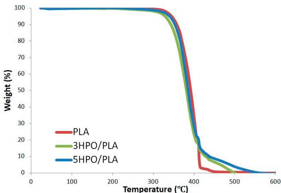
**Figure 3.** TGA thermograms of the PLA, and HPO-loaded PLA electrospun nonwoven fabrics.
