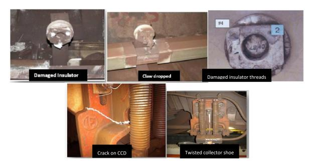
Figure 10. Nature of the damages and structural failures in third rail structure and current collector devices (CCD).
