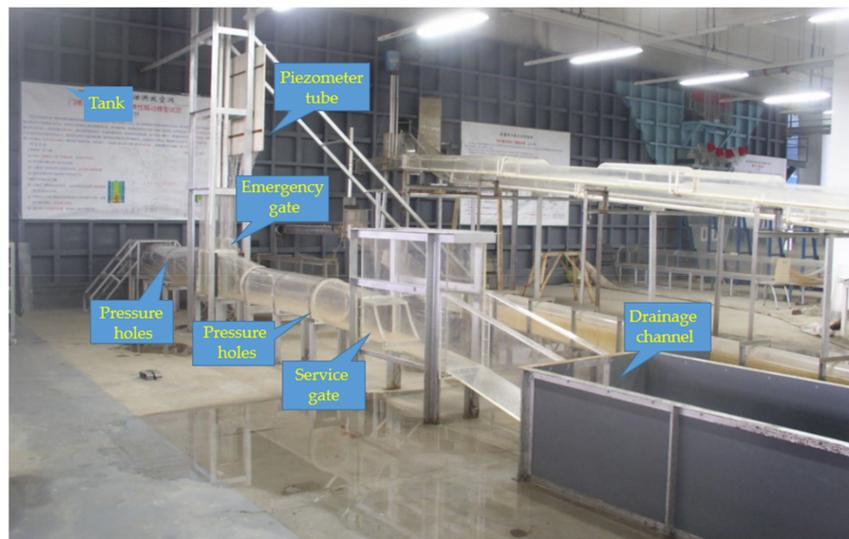
Figure 2. Physical model layout.
