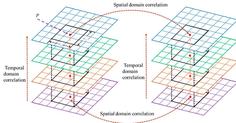
**Figure 3.** Stereo matching based on spatiotemporal correlation. Correlation coefficients are calculated between two cubes composed of correlation windows in the temporal and spatial domains.
