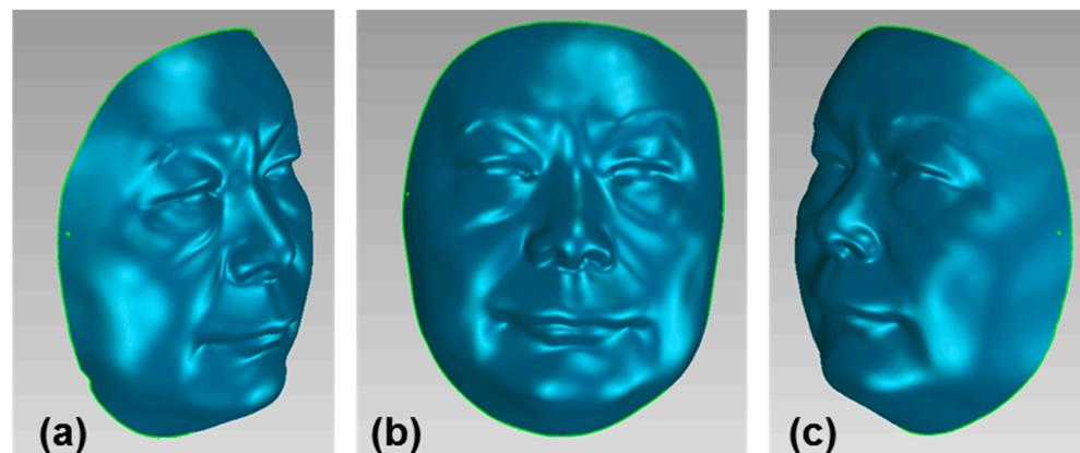
**Figure 10.** Three-dimensional scanned data with ATOS Core 300; (a–c) are different perspectives of the 3D model.
