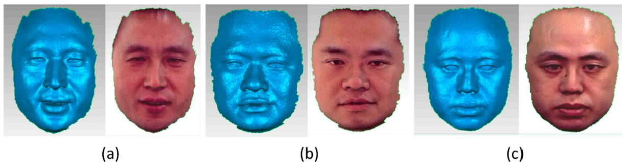
**Figure 15.** (a–c) Three-dimensional reconstruction results of different real faces with N = 12 the speckle stereo image pairs: a contrast display of textured and non-textured maps.
