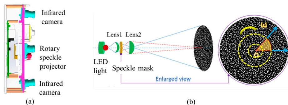
Figure 2. Schematic diagram of 3-dimensional face acquisition device with rotary speckle projector: (a) structure map of the device; (b) internal structure of the rotary speckle projector, where the speckle mask rotates at angular velocity  $\omega$ .
