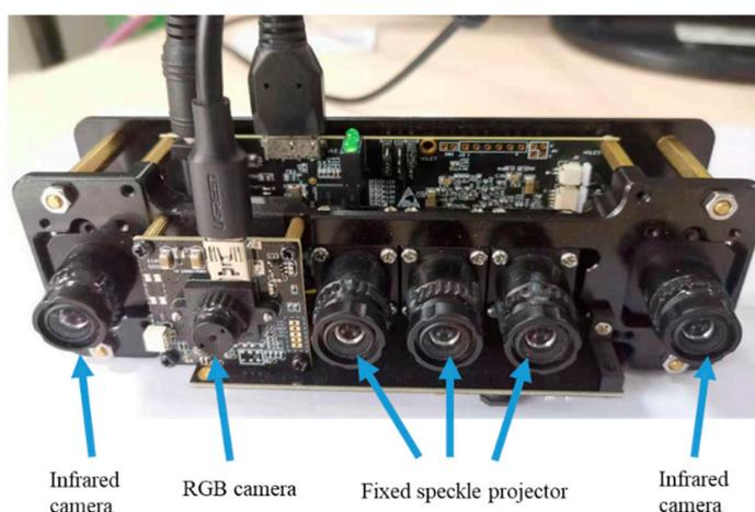
**Figure 8.** Three-dimensional face acquisition device via three fixed-speckle projections.
