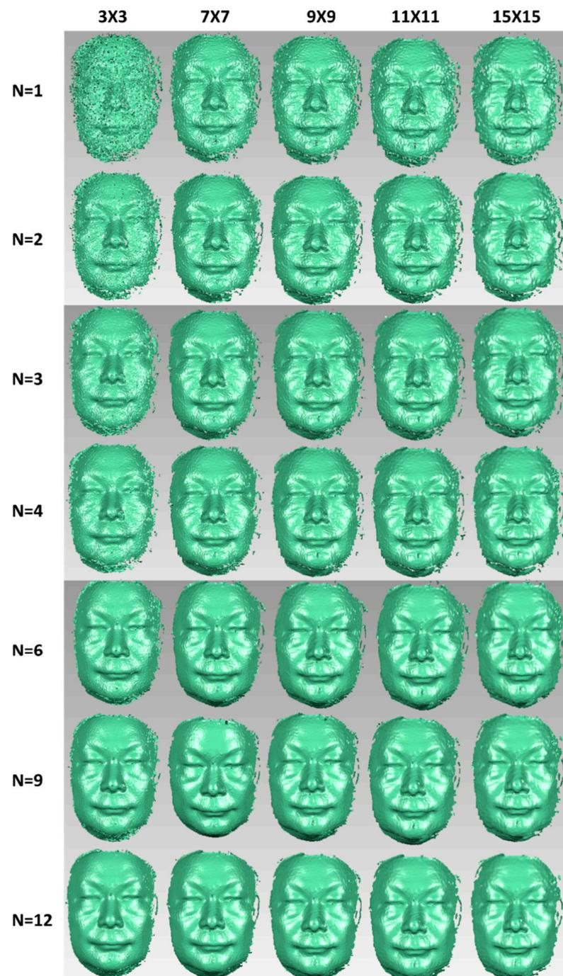
**Figure 11.** Three-dimensional reconstruction results with a number of stereo image pairs,  $N$ , and a fine matching window,  $w_f$ . The reconstruction accuracy continues to improve as  $N$  increases. When  $N$  is small (e.g.,  $N \leq 3$ ), a larger window creates a more precise and complete model.
