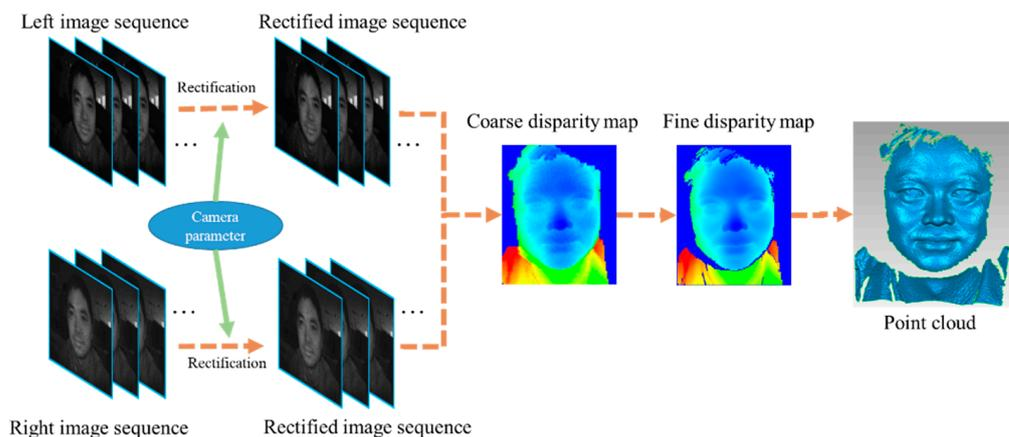
**Figure 4.** Block diagram of the fast stereo-matching method for 3D face reconstruction.
