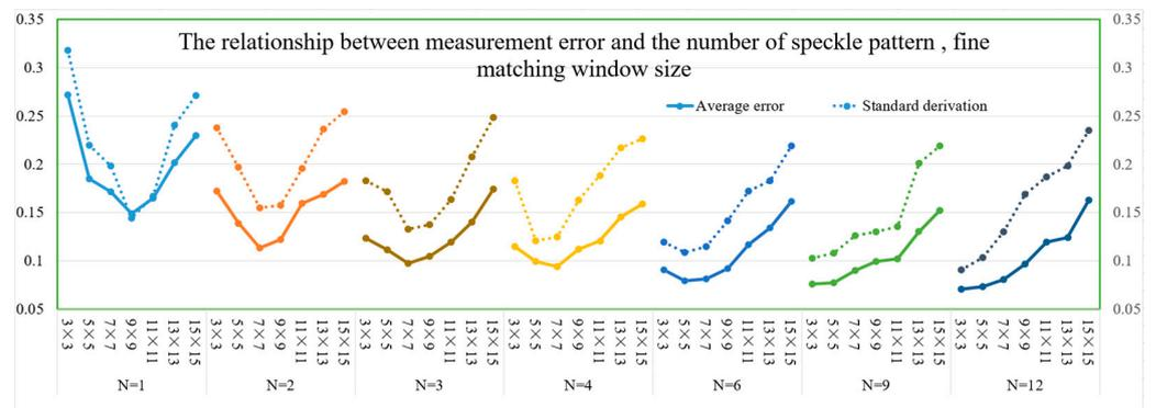
**Figure 12.** Comparison of reconstruction error obtained between the projected pattern numbers,  $N$ , and fine matching window,  $w_f$ . When  $N$  continues to increase, the reconstruction error decreases accordingly. Meanwhile, the optimal window size will also drop.
