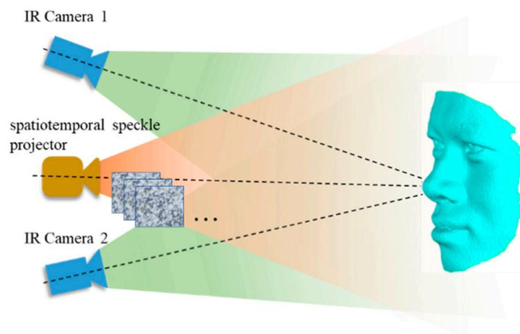
Figure 1. Spatiotemporal stereo scheme for fast three-dimensional face reconstruction.
