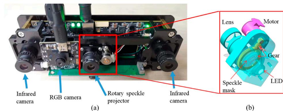
**Figure 7.** (a) Three-dimensional face acquisition equipment with rotary speckle projector. (b) Internal structure diagram of rotating speckle projector.
