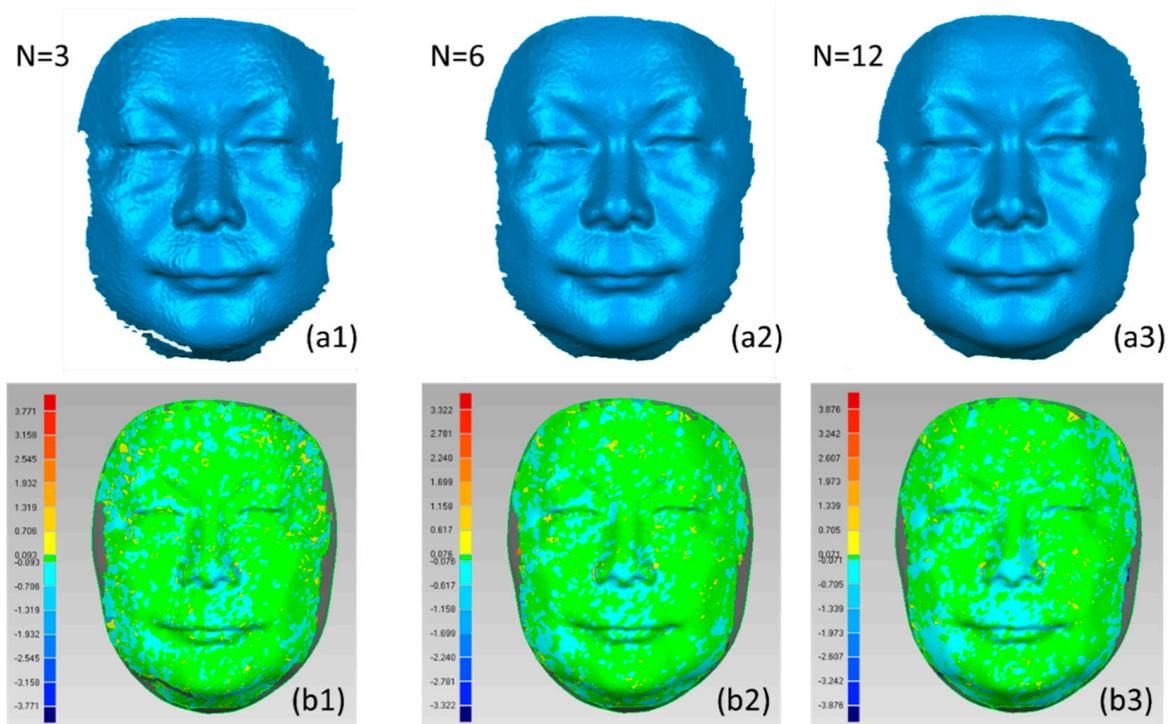
**Figure 14.** (a1–a3) Three-dimensional (3D) reconstruction results of (N = 3, 6, 12) different speckle stereo image pairs. (b1–b3) Corresponding comparison maps with 3D scanned data by ATOS Core 300.
