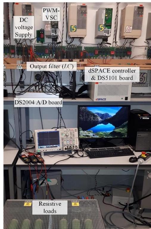
**Figure 2.** Experimental setup to implement the conventional model predictive control (MPC) and the proposed adaptive MPC on a three-phase inductor and capacitor filter (LC)-filtered voltage source inverter (VSI).
