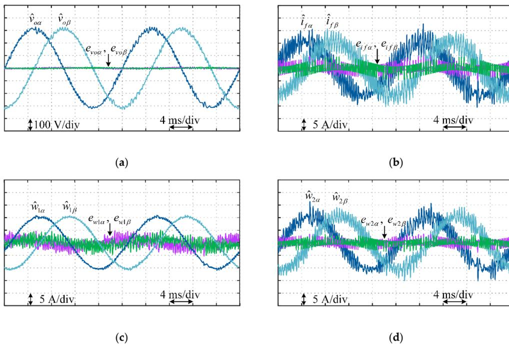
**Figure 7.** Simulation results showing outputs of the proposed adaptive observer under nominal load (5 kW) and 75% error in the initial value of filter capacitance ( $e_C = 75\%$ ), (a) estimated capacitor voltages and voltage estimation errors (b) estimated inverter currents and current estimation errors, (c,d) estimated disturbance inputs and disturbance estimation errors.
