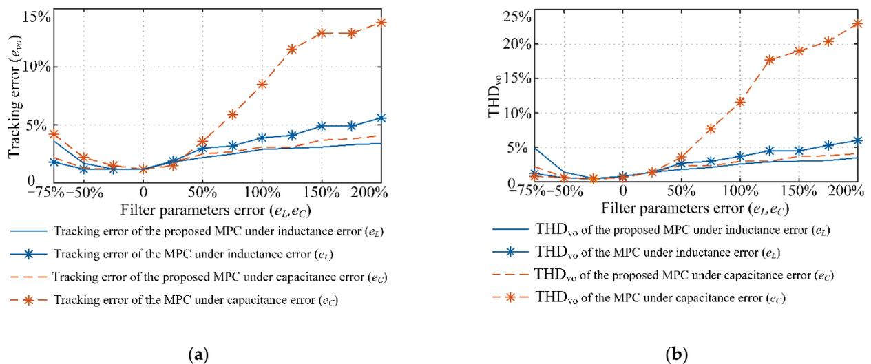
**Figure 8.** Simulation results showing robustness analysis of the proposed adaptive MPC and conventional MPC against the filter parameters uncertainties, (a) voltage tracking error, (b) total harmonic distortion (THD<sub>vo</sub>).
