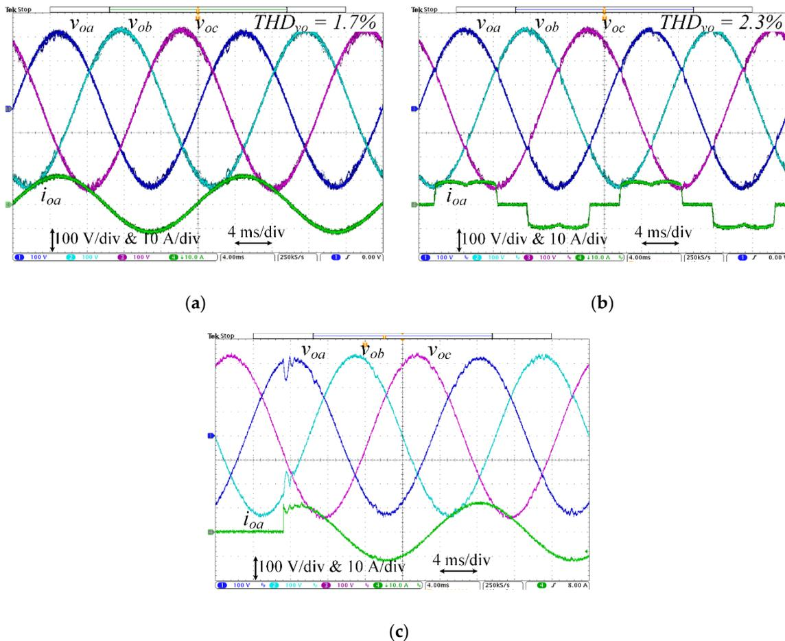
**Figure 9.** Experimental results showing performance of the proposed adaptive MPC under different conditions, (a) and (b) steady-state performance under linear and nonlinear loads, and (c) transient performance under step-change of the load from zero to 5 kW.
