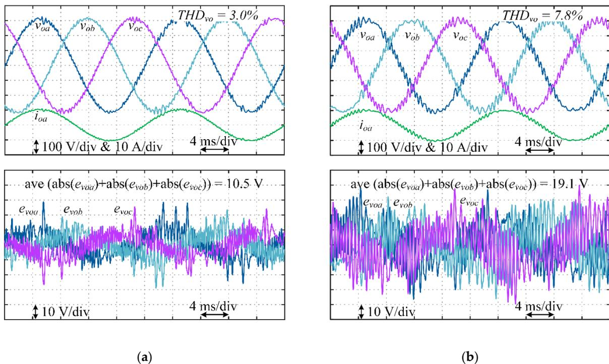
**Figure 6.** Simulation results showing steady-state performance under nominal load (5 kW) and 75% error in the initial value of filter capacitance ( $e_C = 75\%$ ), (a) the proposed adaptive MPC, (b) conventional MPC.
