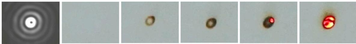
Figure 3. Image of a quasi-Bessel beam formed with a binary axicon and recorded by a microbolometer detector array (compare with Figure 1e). Right: sequence of video frames demonstrating firing paper with this beam. In this case, no polarization converter was used, and the beam had linear polarization. Frame dimensions were  $16.32 \times 12.24 \text{ mm}^2$ .
