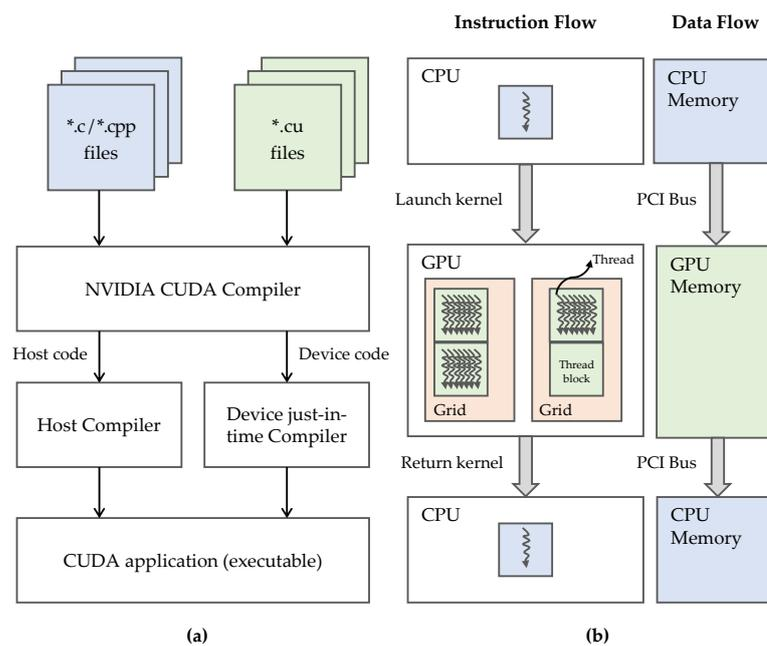
**Figure 1.** (a) Compilation process of CUDA C/C++ sources; (b) CUDA instructions and data flow at runtime.
