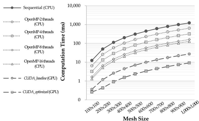
**Figure 9.** Average objective function computation time of sequential CPU, multi-threaded CPU, and parallel GPU implementations.
