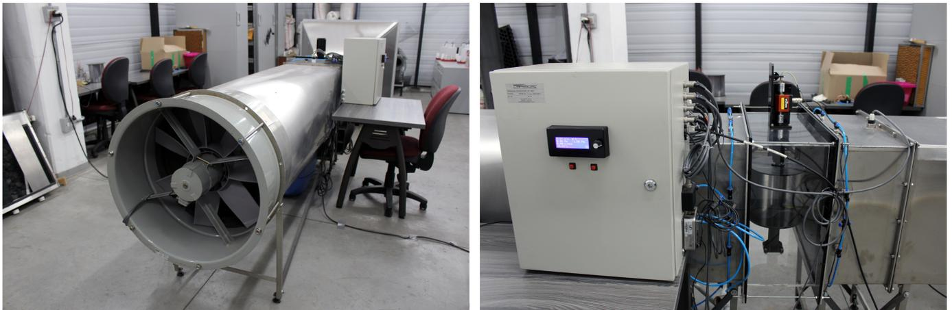
**Figure 10.** Wind tunnel used for experimental development (left). Detail of the experimental setup and the measurement system (right).
