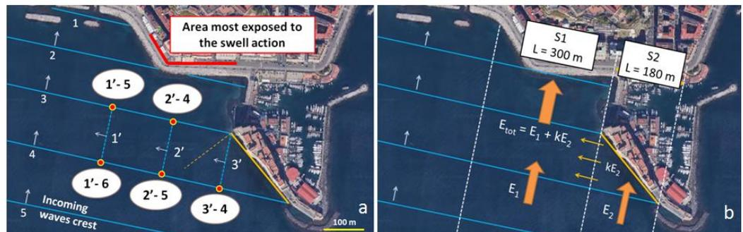
**Figure 18.** Complex scenario of wave motion in front of Via Partenope, due to the reflection of incident waves on the western bastion of Castel dell'Ovo. Reflected waves are indicated with dotted light blu lines 1'-2'-3' (a). (b) The energy flux reflected by Castel dell'Ovo, enhances the wave energy impacting Via Partenope. Equation indications are from Equation (20).
