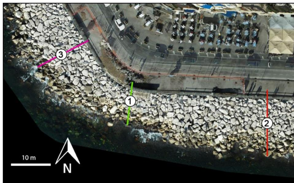
**Figure 22.** Reduction in width of the seawall, with a maximum in correspondence of the bend of Via Partenope Street (Section 1). The three section profiles are shown in Figure 23.
