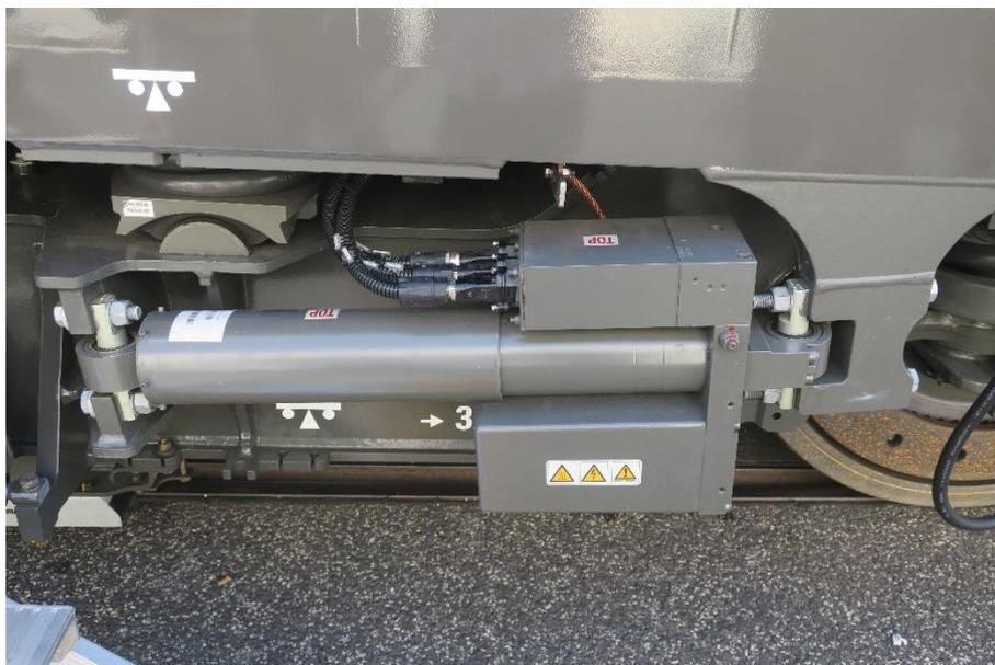
**Figure 1.** Active yaw damper on Siemens Vectron MS locomotive for ÖBB, Inntrans fair 2018.
