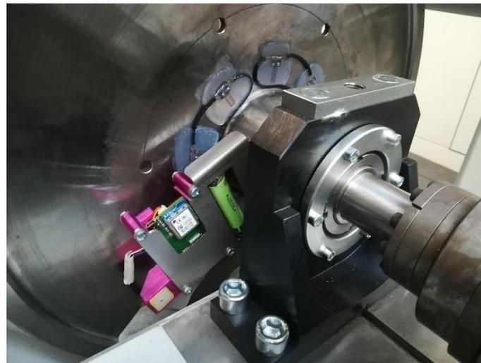
**Figure 15.** Strain gauge instrumented roller with wireless transmitter module.
