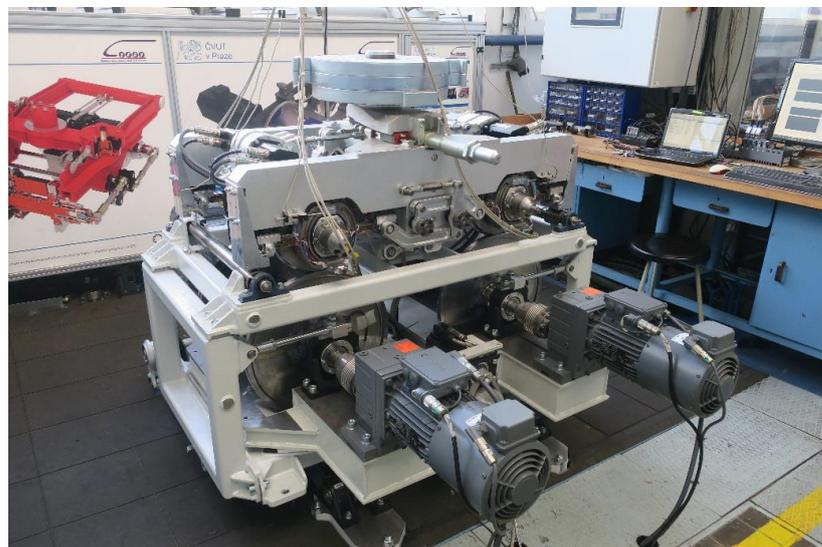
**Figure 5.** Scaled roller rig of the Czech Technical University.
