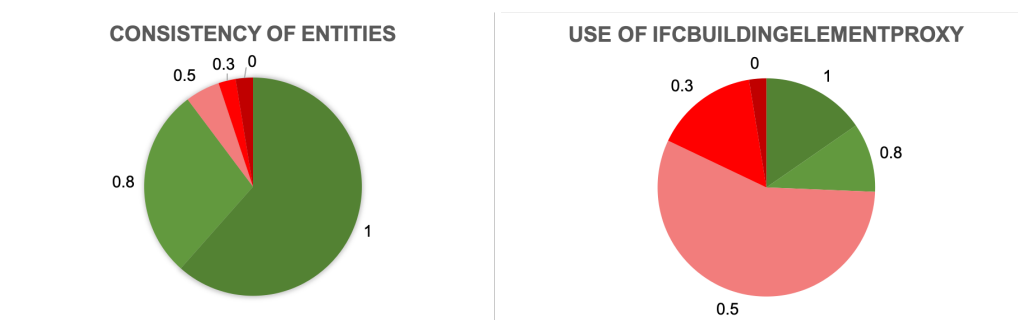
Figure 5. Distribution of models according to the assigned score about the consistency of entities and use of IfcBuildingElementProxy .
