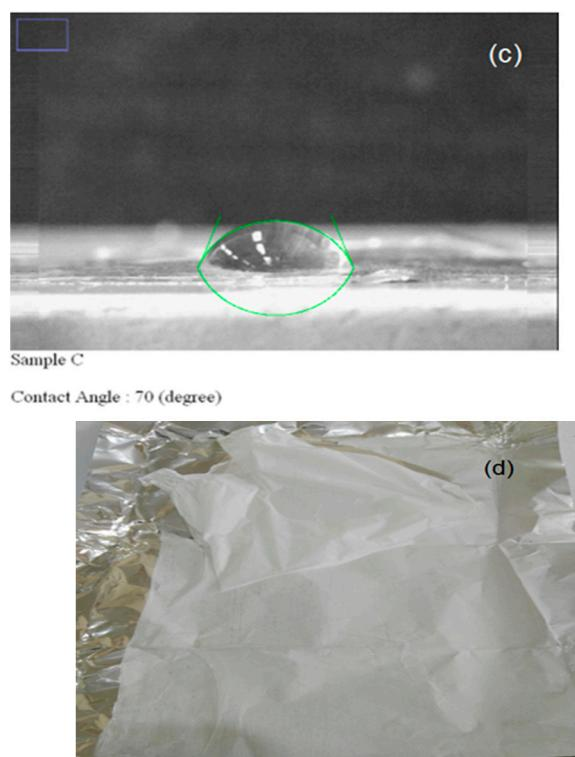
**Figure 4.** (a) SEM images, (b) fiber diameter distribution, (c) contact angle, (d) the image of Bup/PVP/PVA nanofiber.
