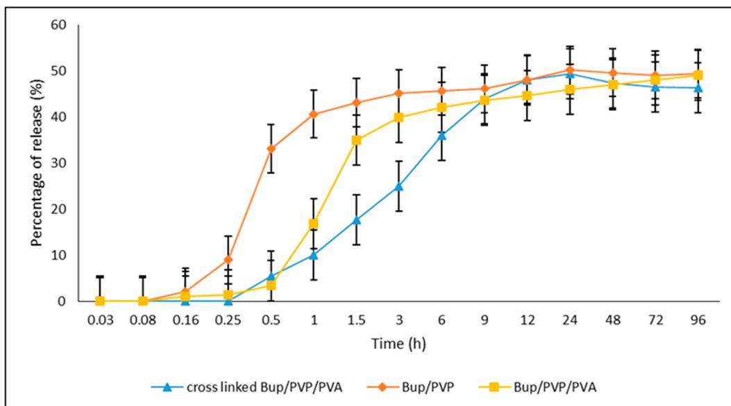
**Figure 11.** The buprenorphine release profile of electrospun drug-loaded nanofiber mats (900 mL phosphate buffered saline, 100 rpm, 37 °C).
