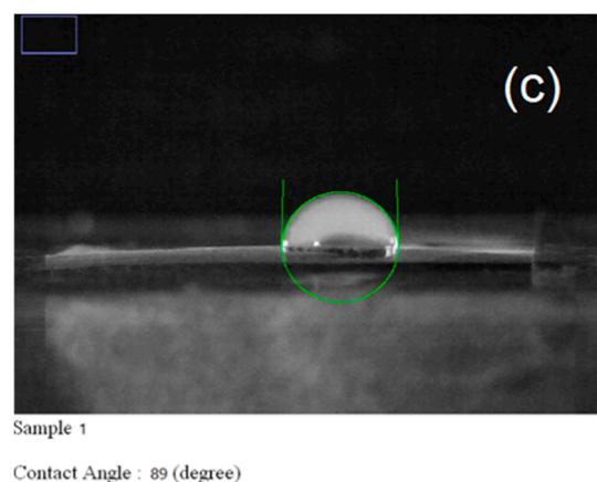
**Figure 1.** (a) Scanning electron microscope (SEM) images, (b) fiber diameter distribution, (c) the contact angle of PVP nanofibers.
