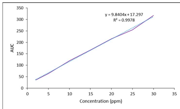
**Figure 10.** Calibration curve of Bup standard solutions in PBS.
