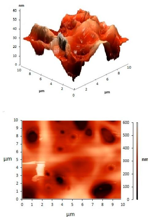
**Figure 8.** Atomic force microscopy (AFM) topography image of glutaraldehyde (GTA) cross-linked Bup/PVP/PVA nanofiber mats.
