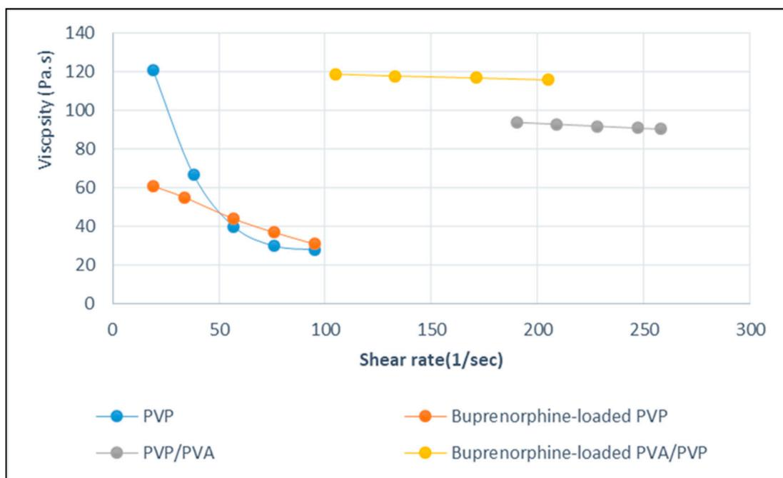
**Figure 5.** Viscosity versus the shear rate of electrospinning solutions.
