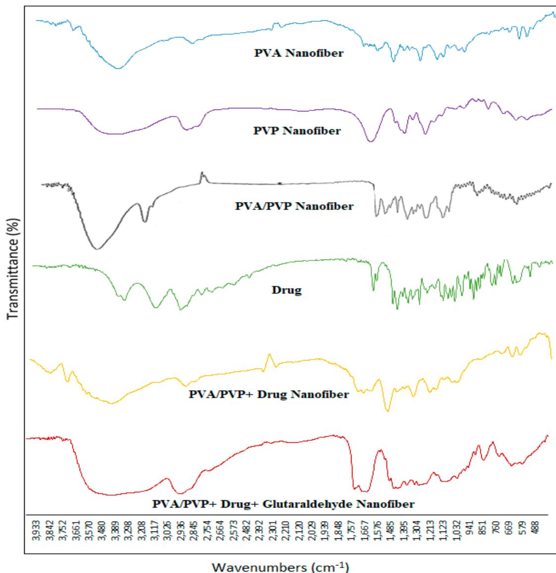
**Figure 7.** Fourier transform infrared (FT-IR) spectra of PVA nanofibers, PVP nanofibers, PVA/PVP nanofibers, Bup, Bup/PVP/PVA nanofibers and cross-linked Bup/PVP/PVA nanofibers.
