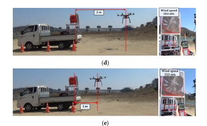
**Figure 12.** This is the wind resistance of the developed drone: (**a**) wind speed of 6.6 m/s at a distance of 8 m from the fan to the drone; (**b**) wind speed 7.7 m/s at a distance of 6 m from the fan to the drone; (**c**) wind speed 8.7 m/s at a distance 4 m from the fan to the drone; (**d**) wind speed 10.1 m/s at a distance 2 m from the fan to the drone; (**e**) wind speed 12.1 m/s at a distance 1 m from the fan to the drone.
