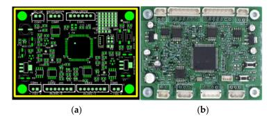
**Figure 5.** This is a VDM of the vehicle detection module part: (**a**) VDM hardware (H/W) artwork; (**b**) Developed VDM.
