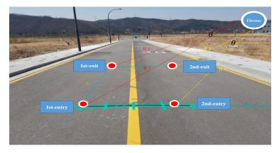
Figure 10. Vehicle detection experiment method on the first and second lines.
