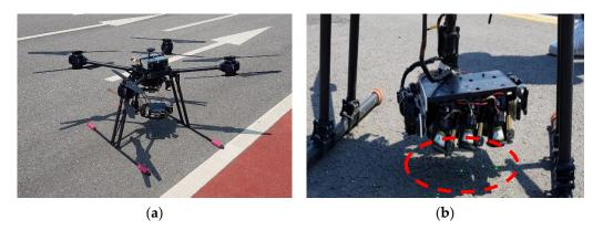
**Figure 9.** This is a developed drone for vehicle detection a lane: (**a**) drone with detection sensor part; (**b**) drone VDM indicating in the red circle.
