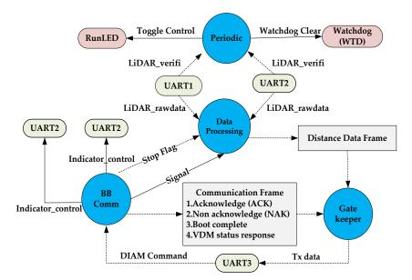
Figure 4. Vehicle detection module (VDM) data flow diagram.
