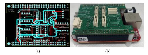
**Figure 6.** This is a detection information acquisition module (DIAM) of the vehicle detection module part: (**a**) DIAM H/W artwork; (**b**) Developed DIAM.
