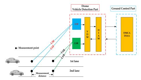
**Figure 2.** Vehicle information acquisition system: LSF—LiDAR sensor front; LSR—LiDAR sensor rear; VDM—Vehicle detection module; DIAM—Detection information acquisition module; DMCA—Detection module control analysis; DIAA—Detection information acquisition analysis.
