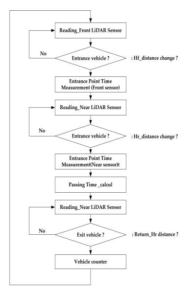
Figure 8. Vehicle measurement time flow chart.
