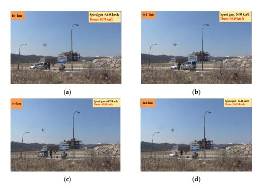
**Figure 11.** Vehicle speed experiment method on the first and second lanes; (**a**) speed gun 58.28 km/h and drone 58.70 km/h on the first lane; (**b**) speed gun 54.83 km/h and drone 55.49 km/h on the second lane; (**c**) speed gun 60.99 km/h and drone 63.15 km/h on the first lane; (**d**) speed gun 53.14 km/h and drone 56.34 km/h on the second lane.
