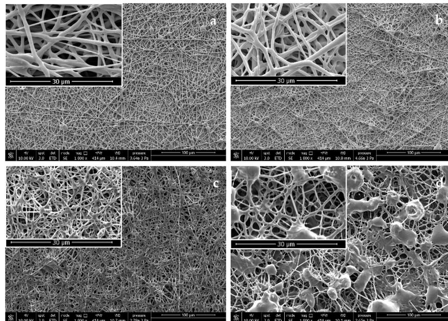
**Figure 2.** SEM micrographs of electrospun PHA fibers: (a,b) PHBHV (commercial), and (c,d) PHB/PHOHD (from Roy's laboratory); (a,c) plain PHAs, and (b,d) PHAs incorporating OLE. Original magnification 1000 $\times$  (scale bar 100  $\mu$ m). Lens show details of the fibers (scale bar 30  $\mu$ m).
