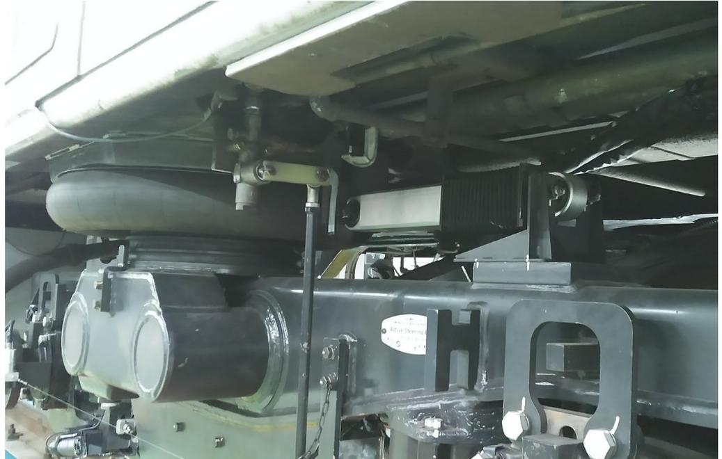
Figure 14. Curvature sensor installed in the test vehicle.
