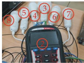
Figure A2. Photo of experimental setup for the reactive power provided by LED devices analysis.
