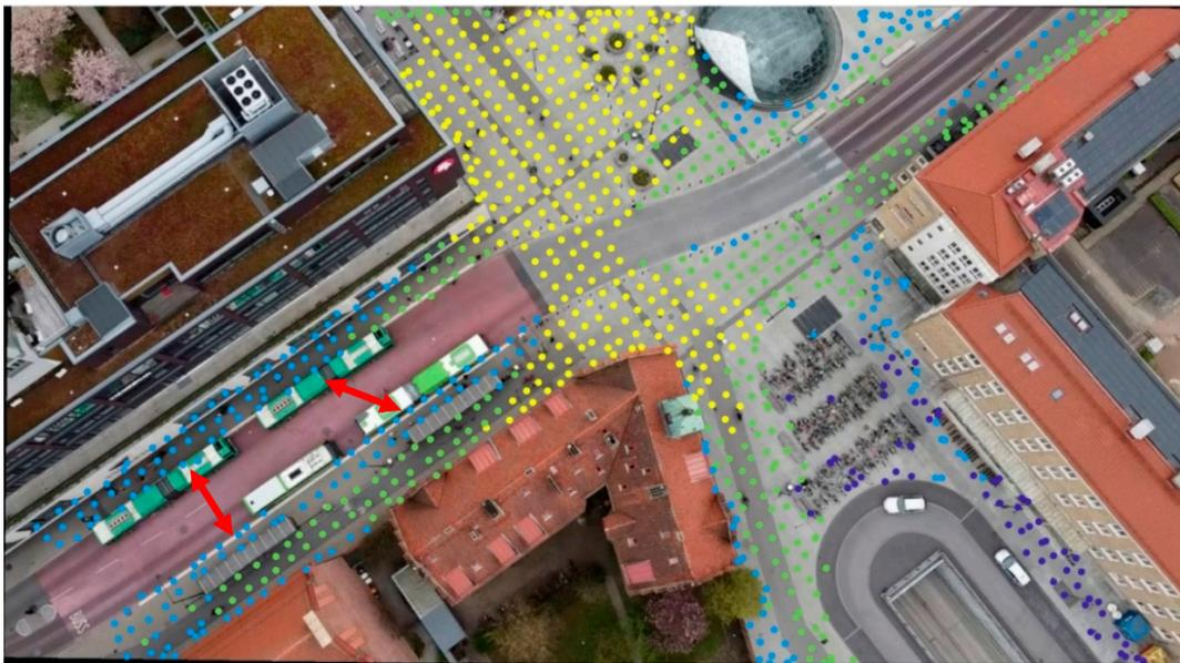
**Figure 9.** One of the camera views at Triangeln showing integration level levels (yellow, green, light blue and dark blue). The red arrows point towards four bus stops which have been included in integration level 3 (light blue).
