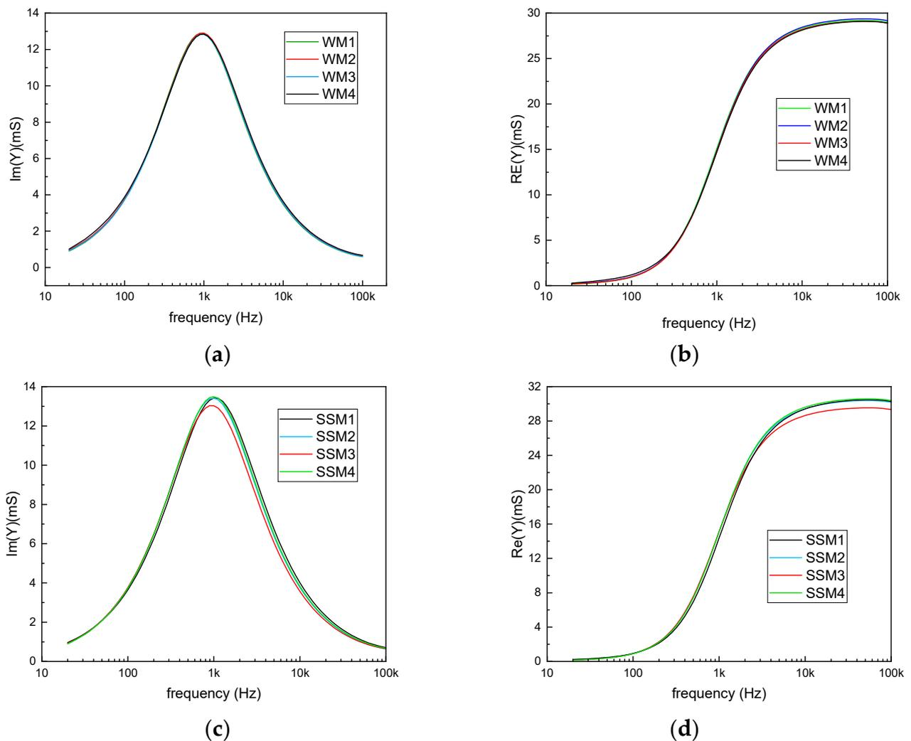
**Figure 3.** (a) Imaginary and (b) real parts of the measured admittances for whole milk samples from different brands; (c) imaginary and (d) real parts of the measured admittances for semi-skimmed milk samples from different brands.
