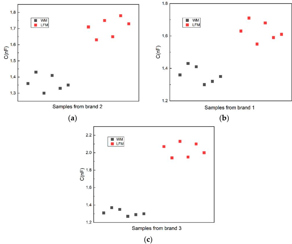
**Figure 8.** Comparison of capacitance values to distinguish whole milk from lactose-free milk for different brands (samples from brand 2 (a); from brand 1 (b) and from brand 3 (c)).
