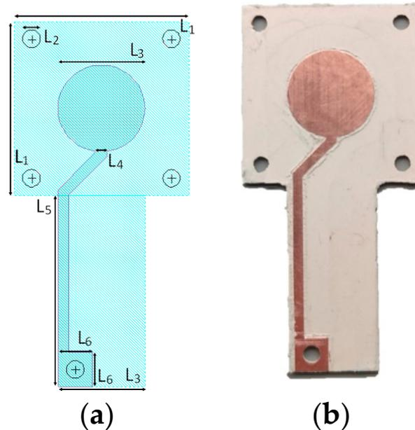
**Figure 1.** The layout (a) and a picture (b) of the electrode employed to perform measurements. The geometry was optimized to reduce parasitic effects.
