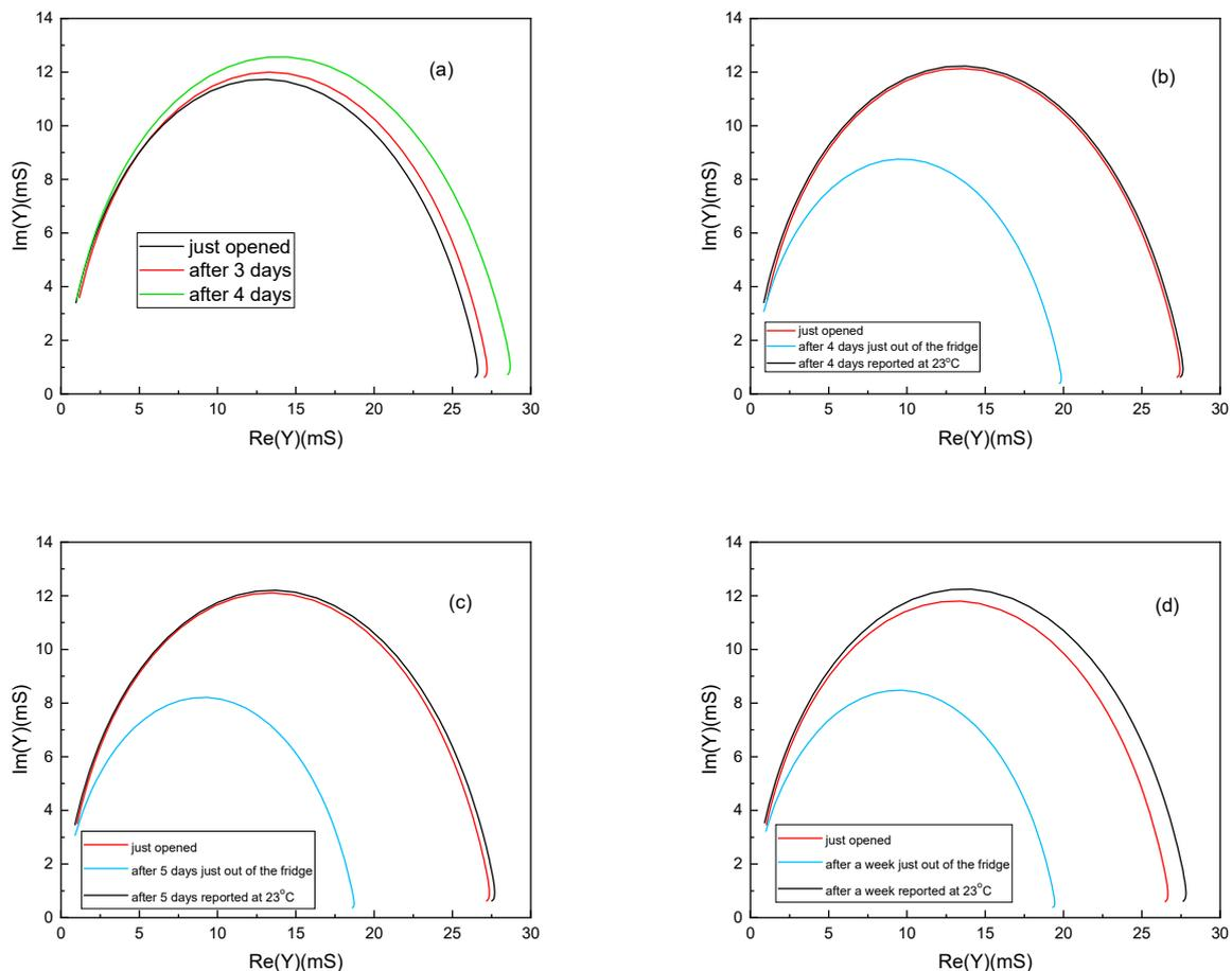
**Figure 12.** (a) variation of the Nyquist diagram of a freshly opened milk sample, after three and four days of storage at room temperature; (b) variation of the Nyquist diagram of a freshly opened milk sample, after 4 days of storage in the fridge as soon as it comes out of the fridge and brought back to room temperature; (c) the same as (b) but after 5 days of storage; (d) the same as (b,c) but after a week of storage.
