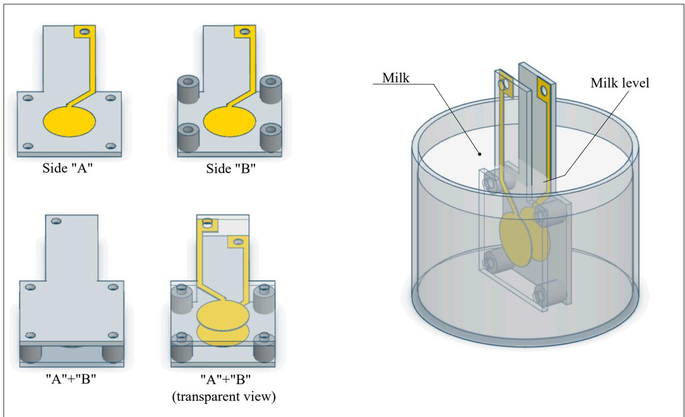
**Figure 2.** Schematic of the assembly of the electrodes and their positioning inside the sample holder. The overlap of the electrodes is performed in such a way as to minimize parasitic capacitive couplings above the milk level.
