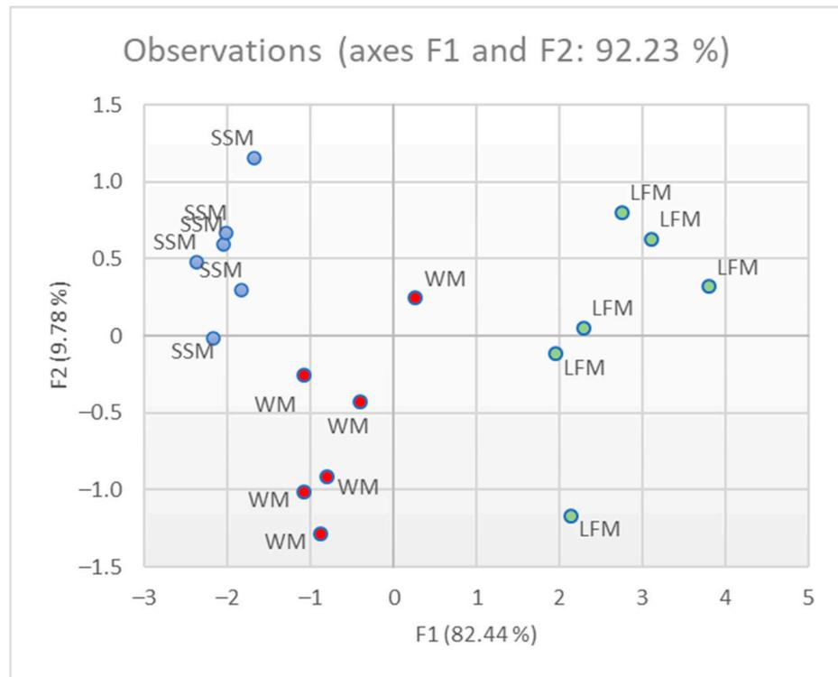
**Figure 10.** PCA analysis to distinguish whole milk (WM, red dots), semi-skimmed milk (SSM, blue dots) and lactose-free milk (LFM, green dots) within brand 1. The PCA has been performed starting from the five variables  $C$ ,  $R$ ,  $Q$ ,  $Im(Y)$  and  $Re(Y)$ .
