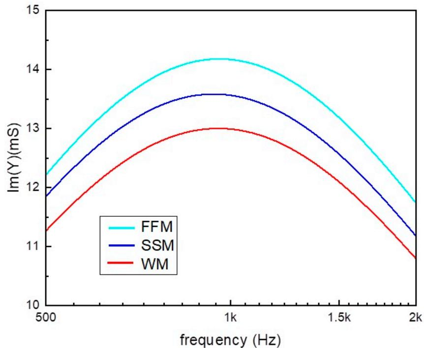
**Figure 5.** Imaginary part of the admittances of different types (whole, semi-skimmed, fat-free) of milk from the same brand. The height of the peak is inversely proportional to the fat content.
