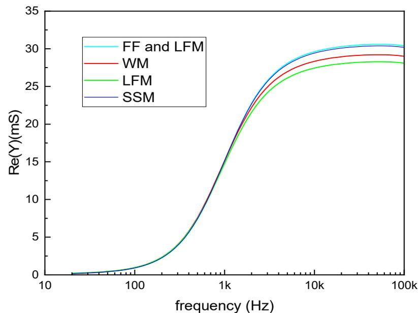
**Figure 6.** Real part of the admittance, that is the conductance, of the same milk samples of Figure 4.
