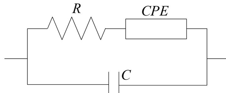
**Figure 7.** Equivalent circuit of milk. The constant phase element (CPE) models the interface electrode/milk; the capacitance  $C$  represents the capacitance of the two electrodes separated by the characterized milk; the resistance  $R$  represents the milk conductance.
