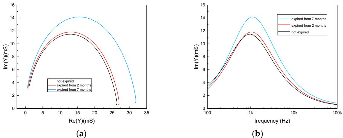
**Figure 13.** Comparison among not expired milk, milk expired from 2 months and milk expired from 7 months. The samples belonged to the same type and brand of milk. In (a) the Nyquist plots are shown, in (b) the Imaginary parts of the admittance, to highlight the modification of the electrical characteristics of expired milk even for frequencies lower than the relaxation frequency of the electrode polarization.
