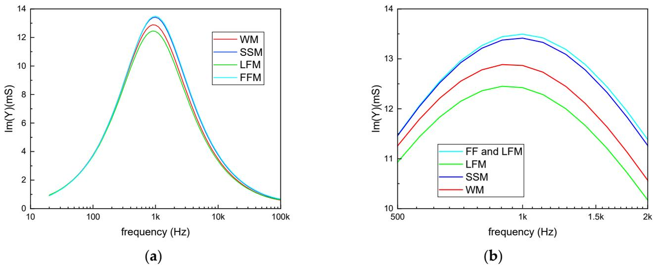
**Figure 4.** (a) Imaginary part of the admittances of different types (whole, semi-skimmed, fat and lactose-free, lactose-free) of milk from the same brand; (b) Detail of Figure 3a.
