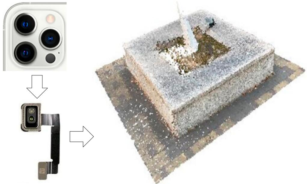
**Figure 4.** The iPhone-based LiDAR sensor and the collected point cloud dataset.
