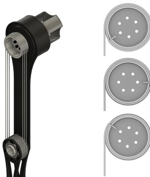
**Figure 5.** The roped transmission structure. The radius does not change in the designed activities.
