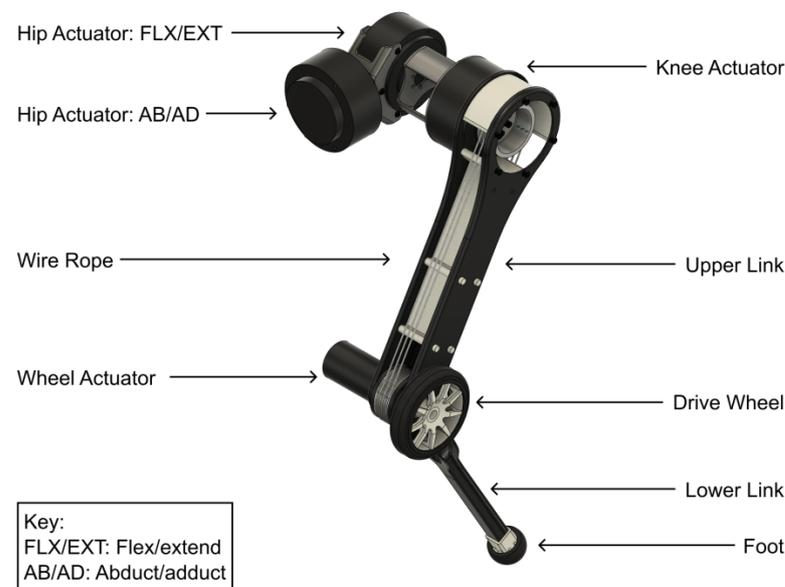
**Figure 3.** The designed structure of a robot leg.
