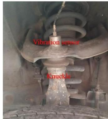
**Figure 2.** The vibration sensor.
