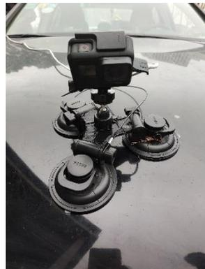
**Figure 3.** The motion camera.
