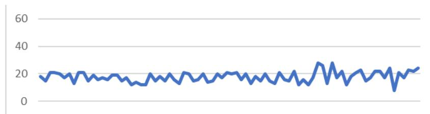
Figure 9. Time delay between CAM message and driver notification on the equipped HMI display in ms.
