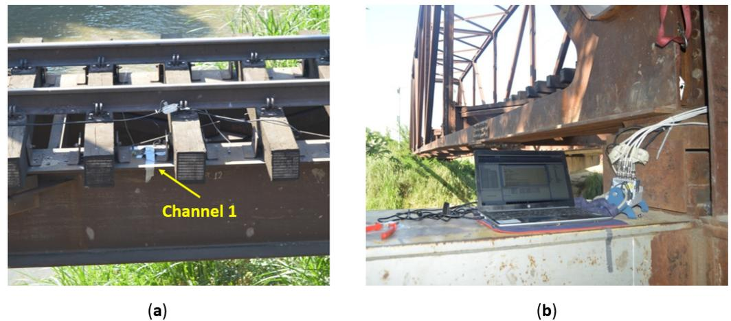
**Figure 10.** Railway bridge monitoring: (a) Location of measurement channel 1. (b) Base station of testing.
