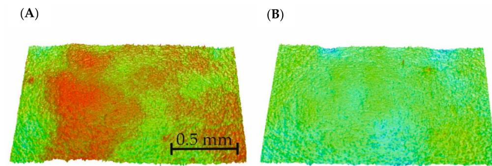
**Figure 6.** Roughness map of the selected samples: (A) non-modified sample (S-0) and (B) sample modified for 10 s (S-10).
