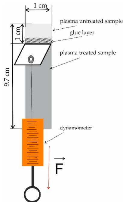
**Figure 2.** Scheme of the adhesive strength test.
