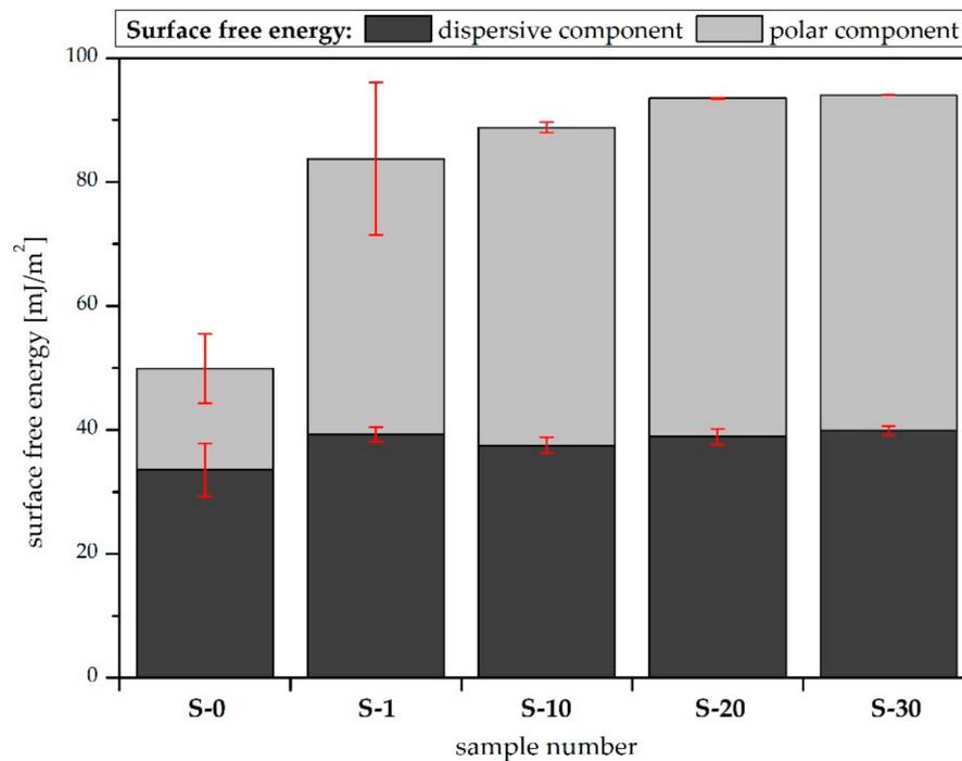
Figure 5. Components of the surface free energy calculated using the LWAB approach.
