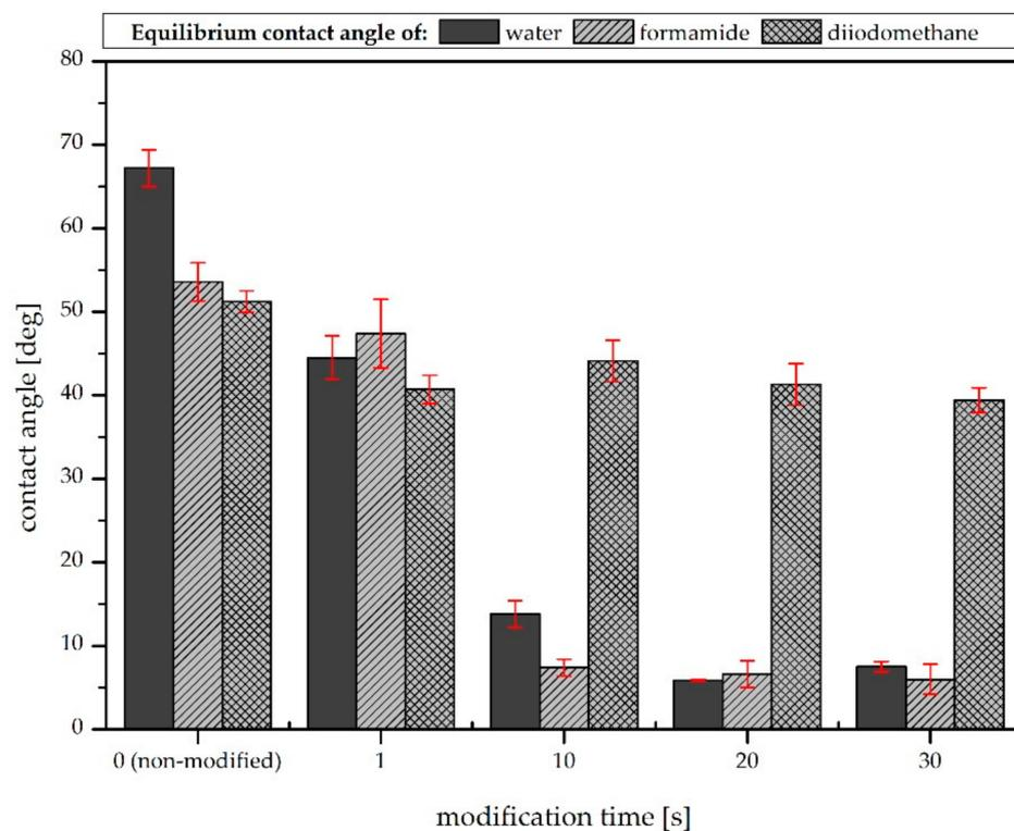
**Figure 3.** Surface wettability (water, formamide, and diiodomethane equilibrium contact angles) versus modification time.
