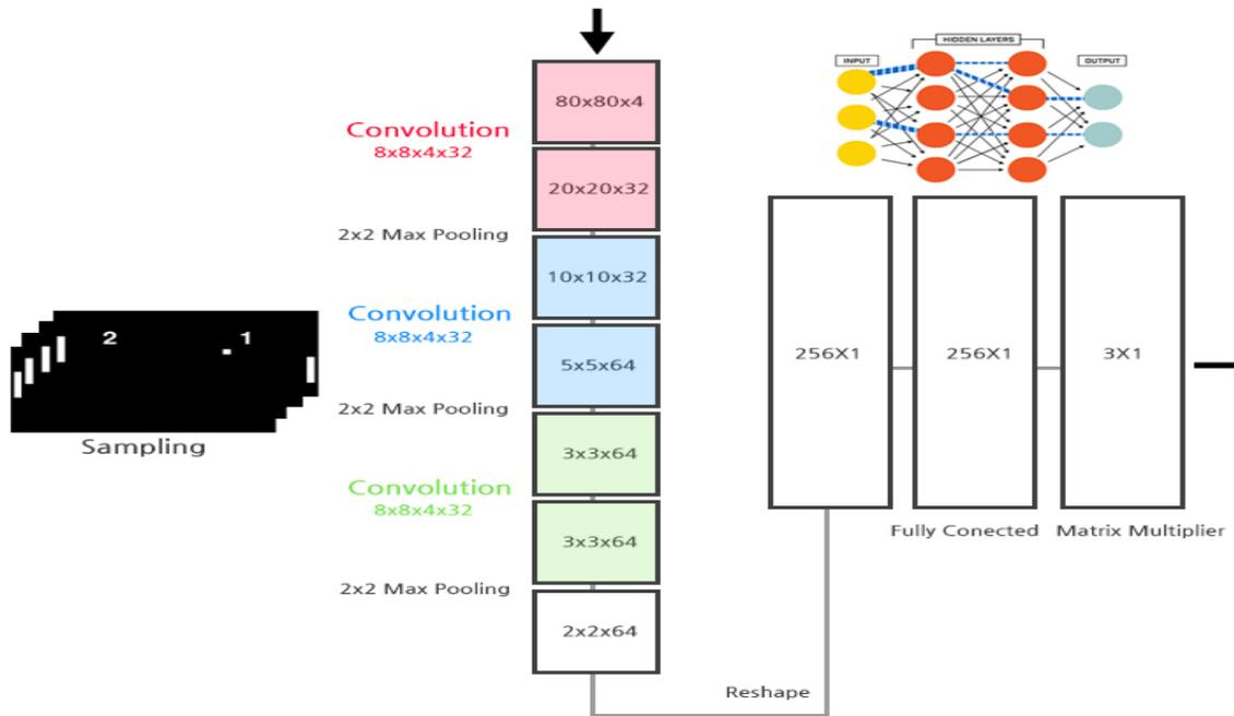
Figure 15. The structure of the implemented artificial neural network.
