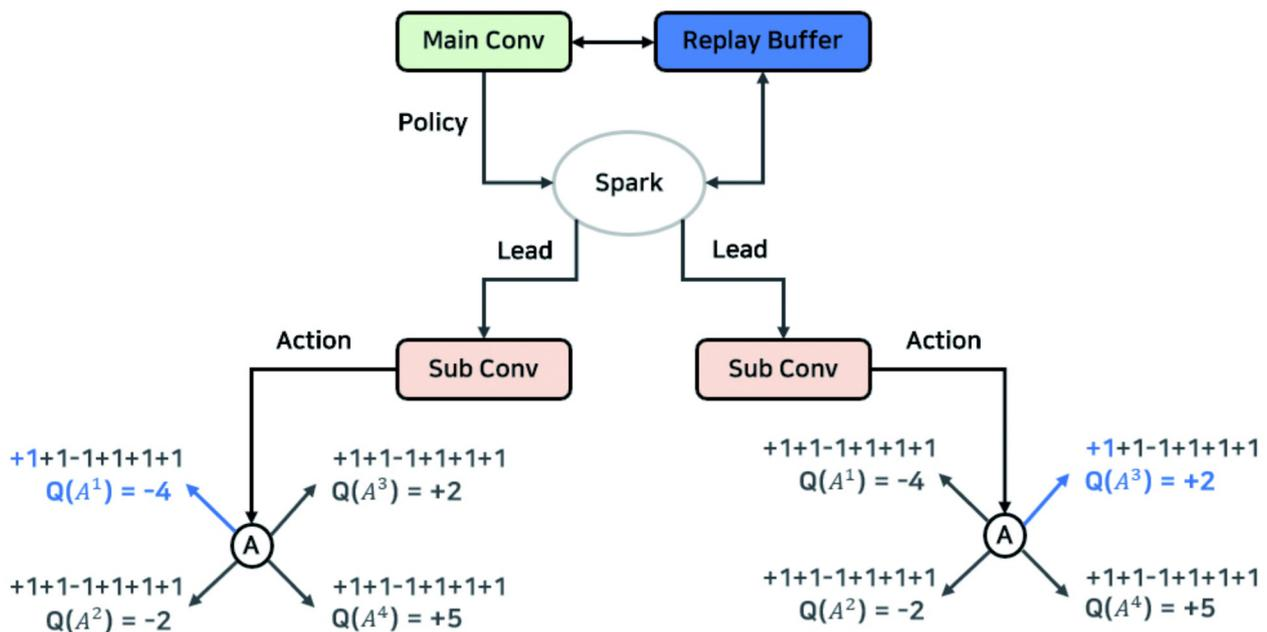
Figure 5. Structure of parallel processing through Spark.
