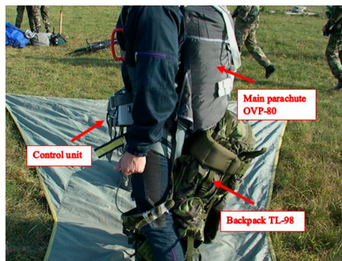
Figure 10. Test skydiver ready to jump (side view; reserve parachute not shown).
