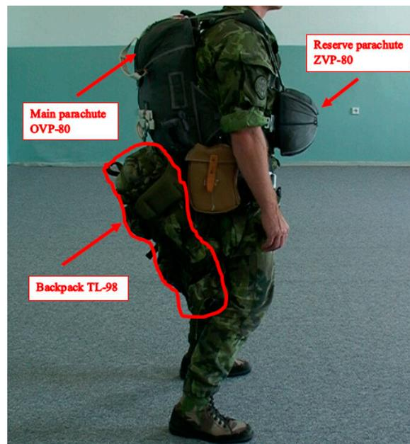
**Figure 2.** Backpack TL-98 fastened to the OVP-80 parachute skydiver harness before jump.
