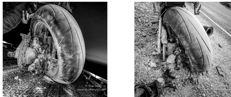
Figure 5. CF wheel failure [14].
