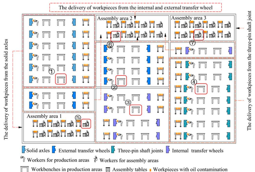
Figure 2. Internal layout of the SDS A3 workshop.
