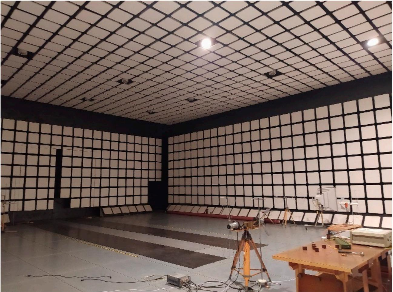
**Figure 2.** An example of anechoic chamber.
