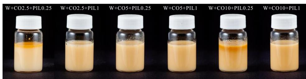
**Figure 1.** The visual appearance of investigated lubricating samples observed half an hour after the preparation.
