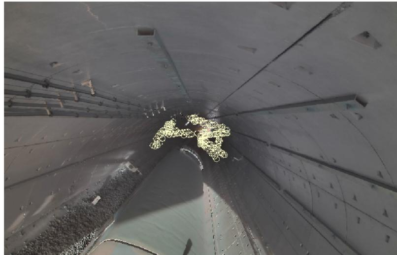
**Figure 20.** Remapping results of contact network frame point cloud and camera image.
