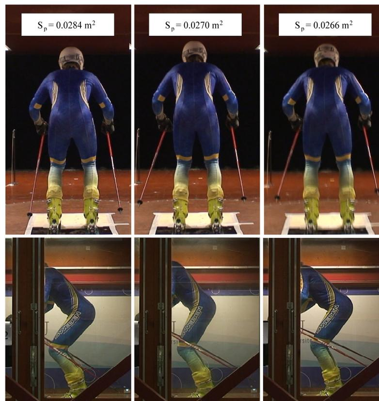
**Figure 3.** The middle position was taken by “Skier 8” during one of the tests at 40 (left), 60 (middle), and 80 km/h (right). At the top is the posterior view and at the bottom is the sagittal view.  $S_p$ —cross-sectional area of the poles.
