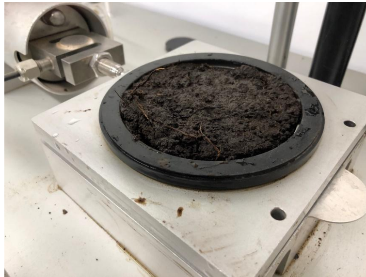
Figure 5. Placement of the test specimen in the Eijkelkamp displacement apparatus.
