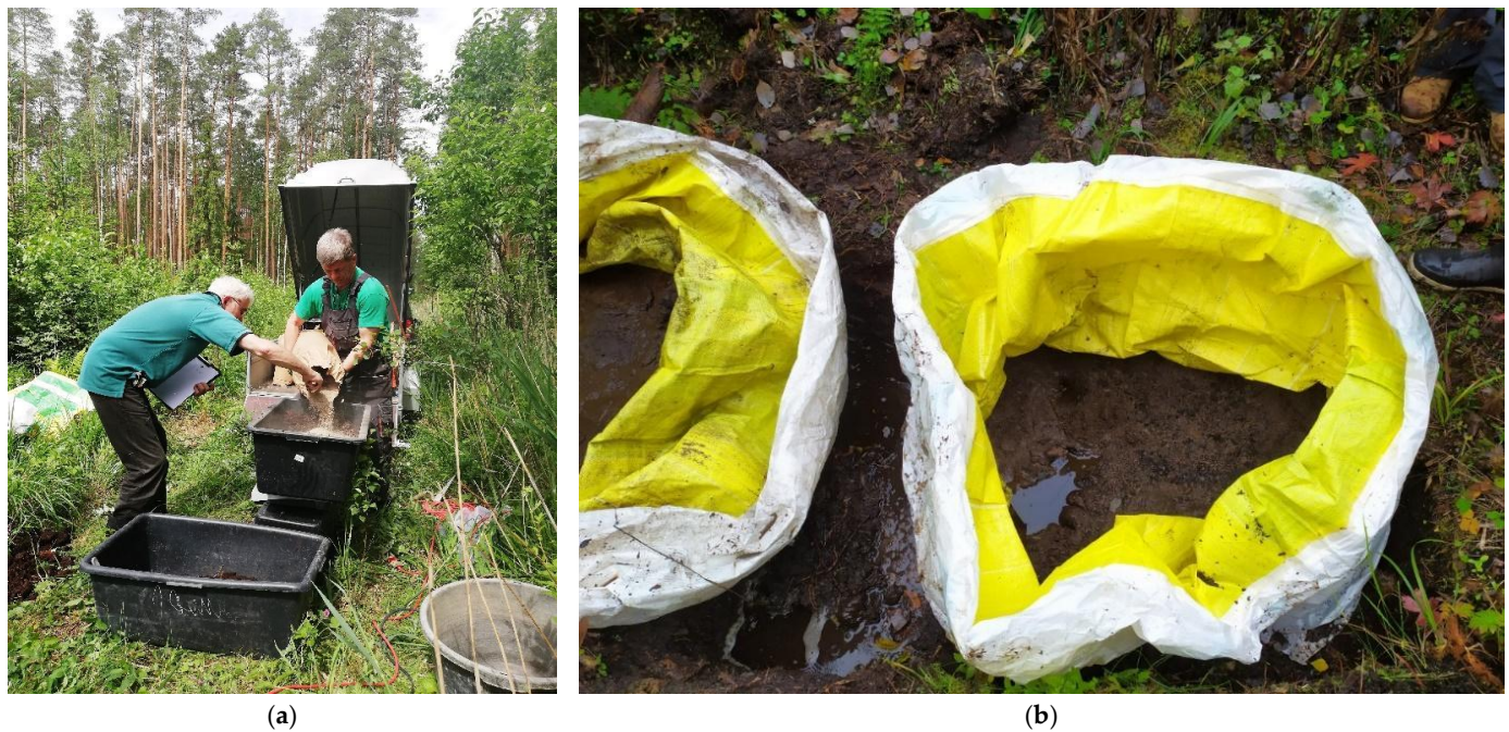
Figure 2. (a) mixing the soil with ash and additives; (b): bigbags partially filled with soil mix (labelled as Bag 1 on the (a) and Bag 2 on the (b)).
