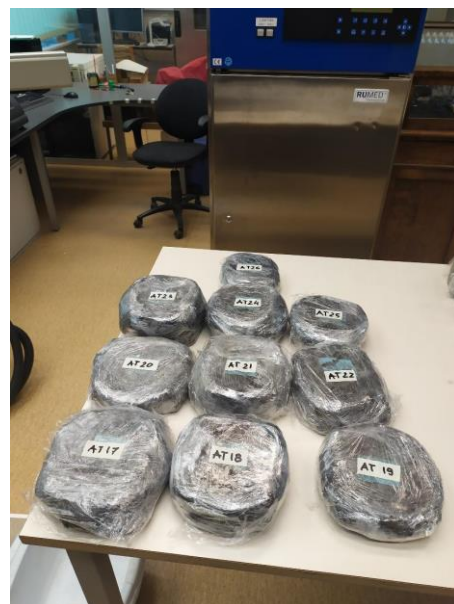
Figure 6. Preparation of specimens for the oedometer tests.
