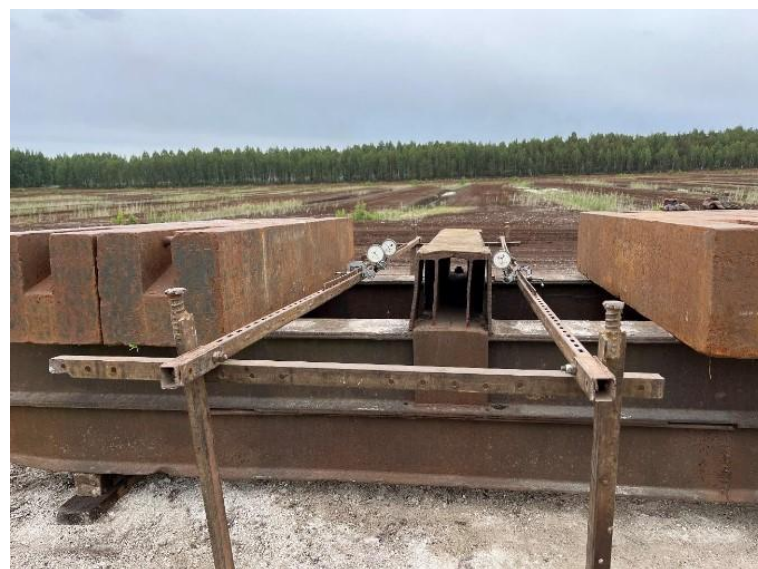
Figure 4. Equipment for the road embankment load test on the test site.
