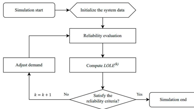
Figure 3. Adequate installed capacity reserve derivation flow chart.
