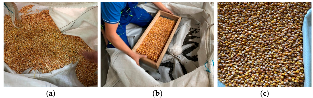
Figure 3. Phases from the separation assessment: (a) corn seeds impurified with sunflower and soybean seeds; (b) manual verification of the separation efficiency; (c) seeds remaining after the separation.
