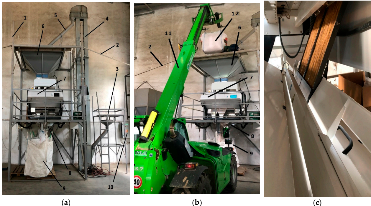
Figure 2. Optical separation of corn seeds: (a) automated feeding using a vertical conveyor; (b) direct feeding with seeds using a front loader; (c) in-depth perspective of the optical separation process. The installation is composed of the following: 1—equipment supporting stand; 2—stiffening beams; 3—feeding stand; 4—vertical conveyor; 5—seed orientation pipe; 6—optical sorter feeding funnel; 7—optical sorter equipment; 8—funnel for big-bag loading; 9—big-bag for seed output; 10—power supply; 11—front loader; 12—big-bag for loading seeds directly using the front loader.
