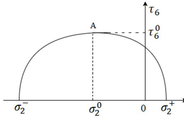
Figure 3. Schematic diagram of the tensile–compressive failure envelope of UD CFRP.
