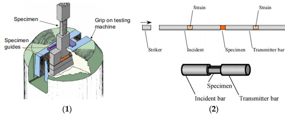
**Figure 4.** Compression testing apparatus: (1) servo-hydraulic machine for intermediate strain rate testing and (2) split Hopkinson bar for high-strain-rate testing [7].
