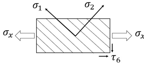
**Figure 1.** An explanation of mechanical properties of UD fiber-reinforced polymers.
