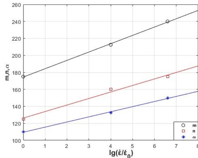
**Figure 7.** Dependence of coefficients  $m$ ,  $n$ ,  $\alpha$  on strain rate (lines—approximation results; points—data from Table 2).
