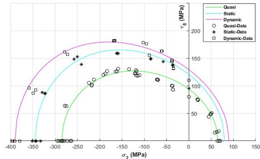
**Figure 5.** Comparison of failure envelopes predicted by MPFE and experimental data at three different strain rates.
