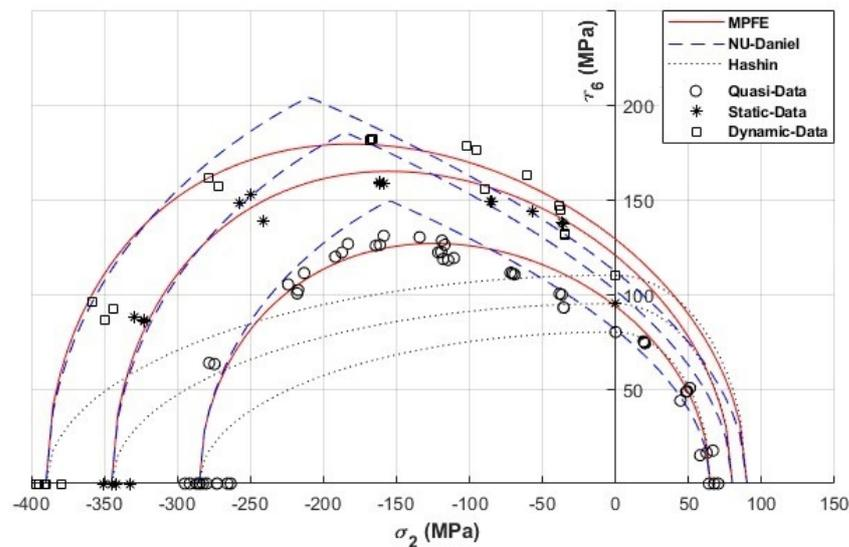
**Figure 6.** Comparison of theoretical failure envelopes for three criteria and the experimental data at three different strain rates.
