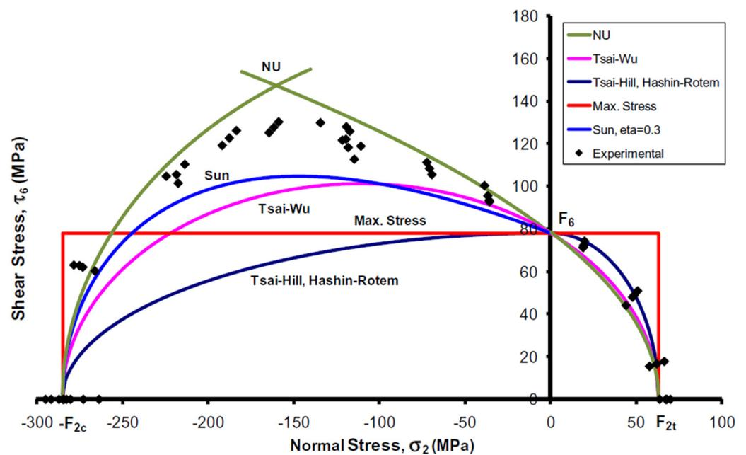
**Figure 2.** Comparison of failure envelopes using different failure criteria and experimental results for UD AS4/3501-6 CFRP under quasi-static transverse normal and shear stress (Reprinted with permission from Ref. [7]. 2011, copyright owner’s Daniel I.M.) [7].
