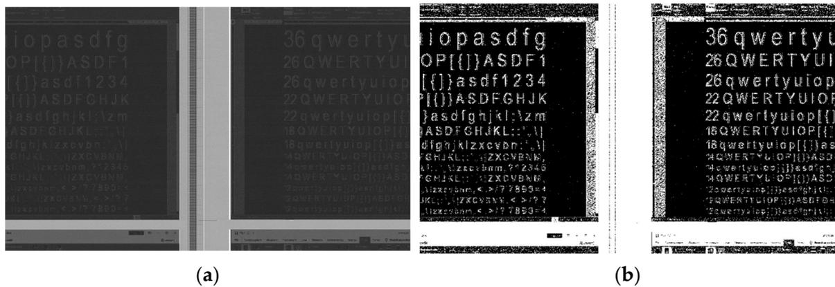
**Figure 5.** Example of (a) an image containing text data reconstructed in electromagnetic infiltration and (b) the same image subjected to pixel amplitude thresholding (pixel amplitude value threshold of 66).
