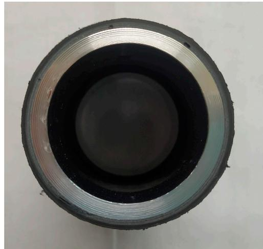
**Figure 15.** Voids in the adhesive joint.
