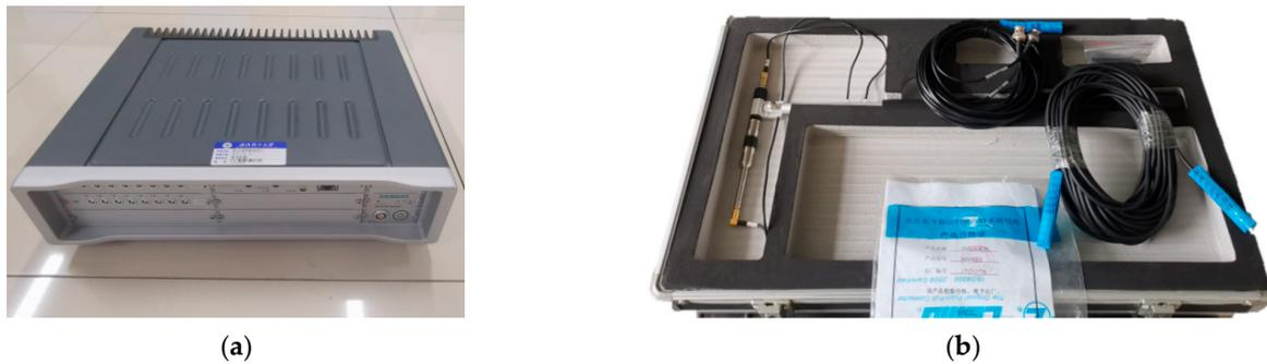
**Figure 1.** Image of the apparatus used in the sound intensity experiment: (a) collector; (b) sound intensity sensor.
