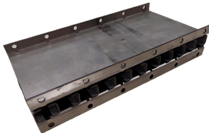
**Figure 2.** Specimen of a reinforced sandwich panel.
