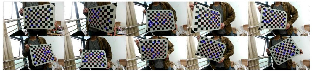
**Figure 13.** Ten images of the calibration plate at different distances and attitudes and the reprojection effects.
