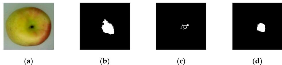
**Figure 11.** Effectiveness of each method for detection of apple stem images. (a) Original figure; (b) genetic algorithm segmentation result; (c) edge detection algorithm result; (d) segmentation effect of the proposed image segmentation method.
