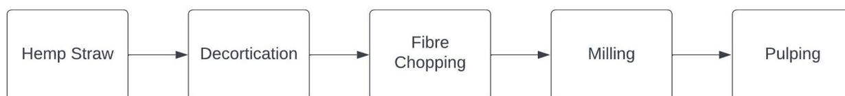
**Figure 9.** Hemp straw processing towards pulp for L-MMCF manufacturing.
