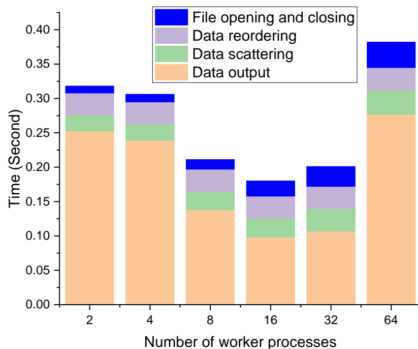
Figure 11. Runtime of outputting a 1D variable at the same I/O primary and worker process.
