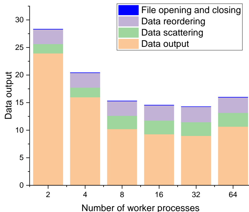
Figure 13. Runtime of outputting a 2D variable along the second dimension at the same I/O primary and worker process.
