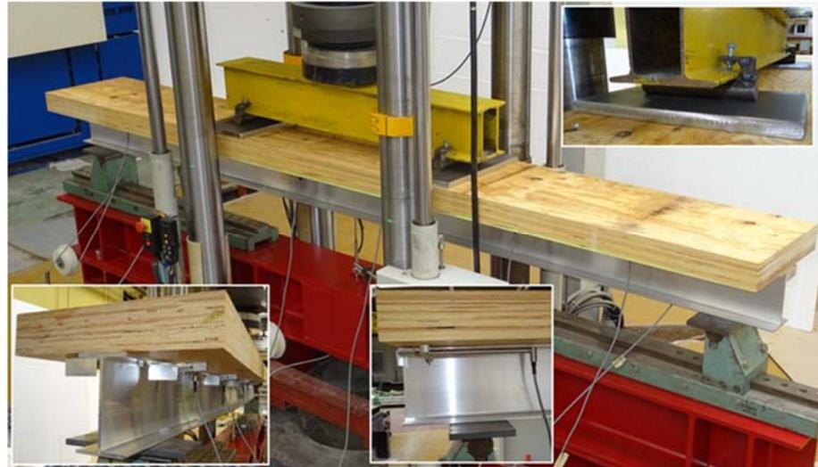
**Figure 1.** Four-point bending test set-up.
