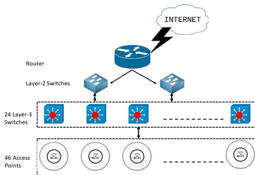
Figure 2. SDN-based architecture.
