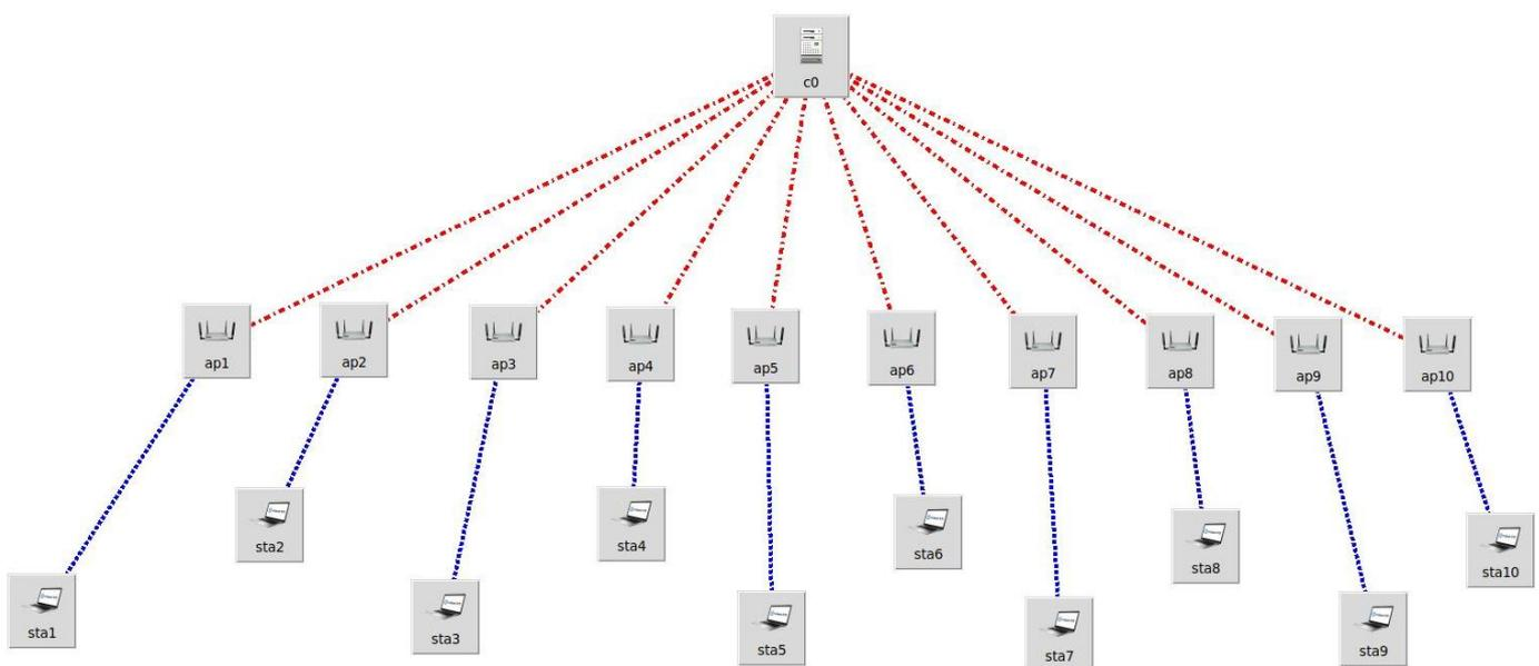
Figure 4. Mininet-Wi-Fi-created linear topology.
