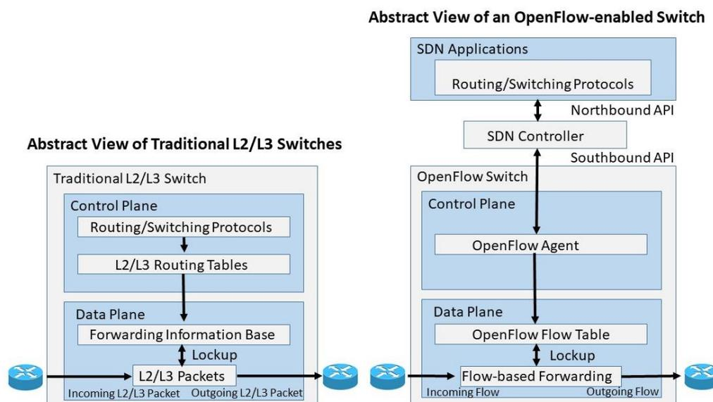
**Figure 1.** The differences between an SDN switch and a traditional switch [17,20,39].
