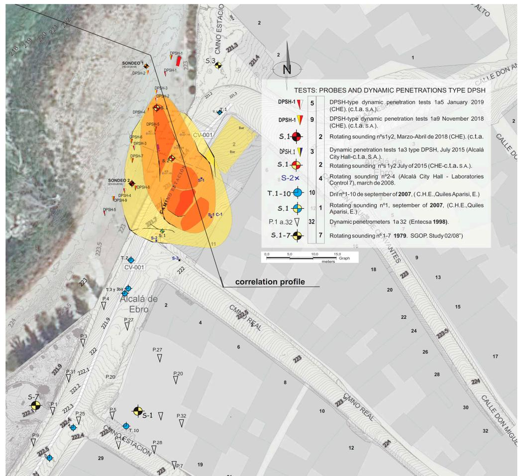
**Figure 3.** Location of the geotechnical investigation works carried out. The areas marked in red indicate sinkholes occurred in the last 15 years. The areas in orange and yellow indicate the contour zones affected by cracks in pavements and buildings, which also show evident signs of subsidence.
