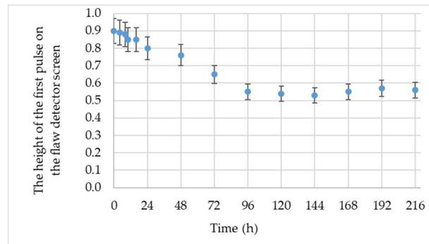
**Figure 13.** Variation in pulse height on the defectoscope screen during non-destructive testing of adhesive bond by ultrasonic Rayleigh surface wave.
