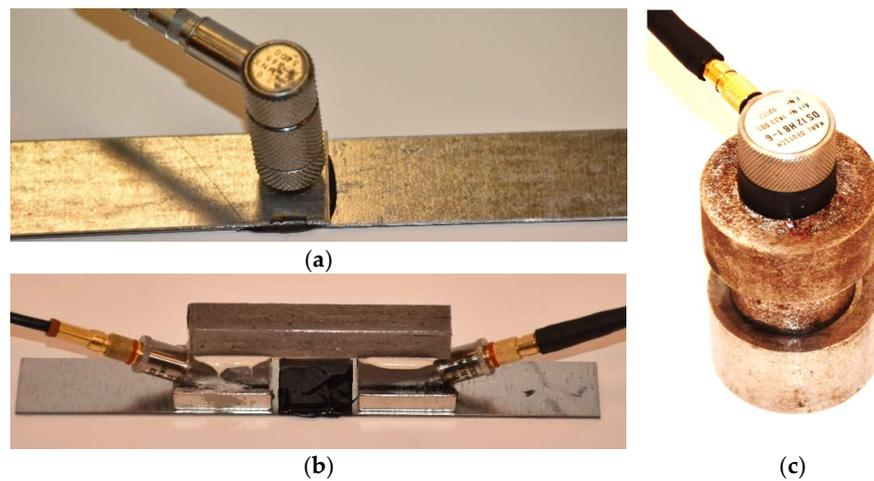
**Figure 8.** Ultrasonic measurement systems: (a) 20 MHz normal wave probe, (b) surface wave probe, and (c) 2.4 MHz normal wave probe.
