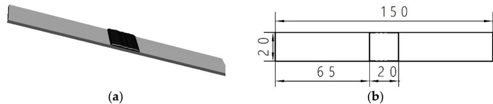
**Figure 6.** Sample used for testing—adhesive applied to the sheet for testing by Rayleigh (surface) wave: (a) a view, and (b) dimensions—in millimeters.
