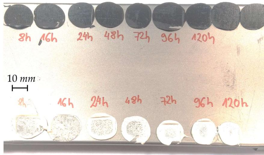
**Figure 3.** A view of the bonds after rupture: indicated times from the formation of each bond to its break for epoxy DP490 3M (**top**) and hybrid Hybrix CX80 Poland (**bottom**) adhesives.
