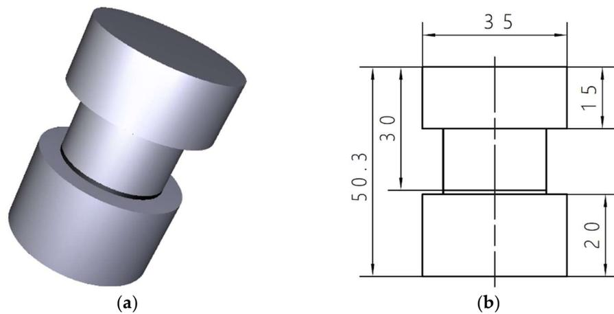
**Figure 5.** Sample used for testing—steel discs for testing by longitudinal wave: (a) a view, and (b) dimensions—in millimeters.
