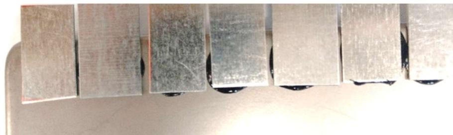
**Figure 2.** An example of samples from the preliminary study (black epoxy adhesive visible DP490 SCOTCH-WELD 3M).
