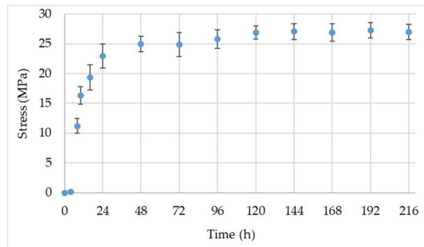
**Figure 14.** The distribution in time of the tensile stresses for connected discs.
