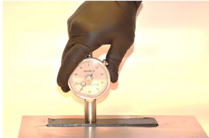
Figure 10. Adhesive hardness test.
