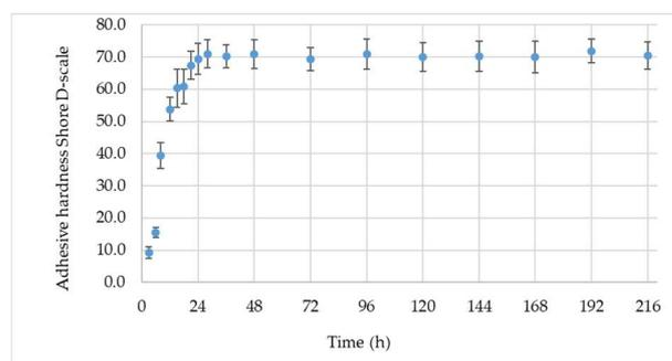
**Figure 18.** The distribution of an adhesive hardness over time.
