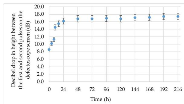
Figure 11. The change in decibel drop between the first and second pulses obtained on the screen of the ultrasonic defectoscope from the bond area for the ultrasonic test of connected steel discs with epoxy adhesive.
