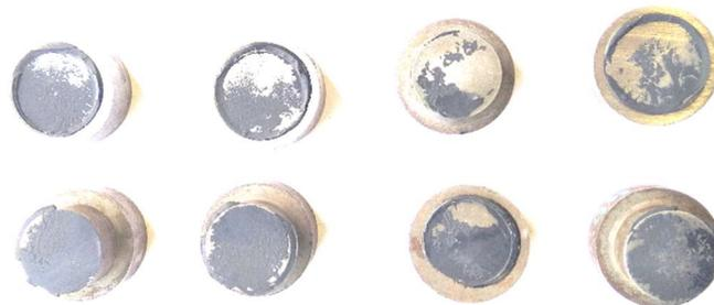
**Figure 16.** An example of a view of the bonded surfaces of the discs after breaking the adhesive bonds.
