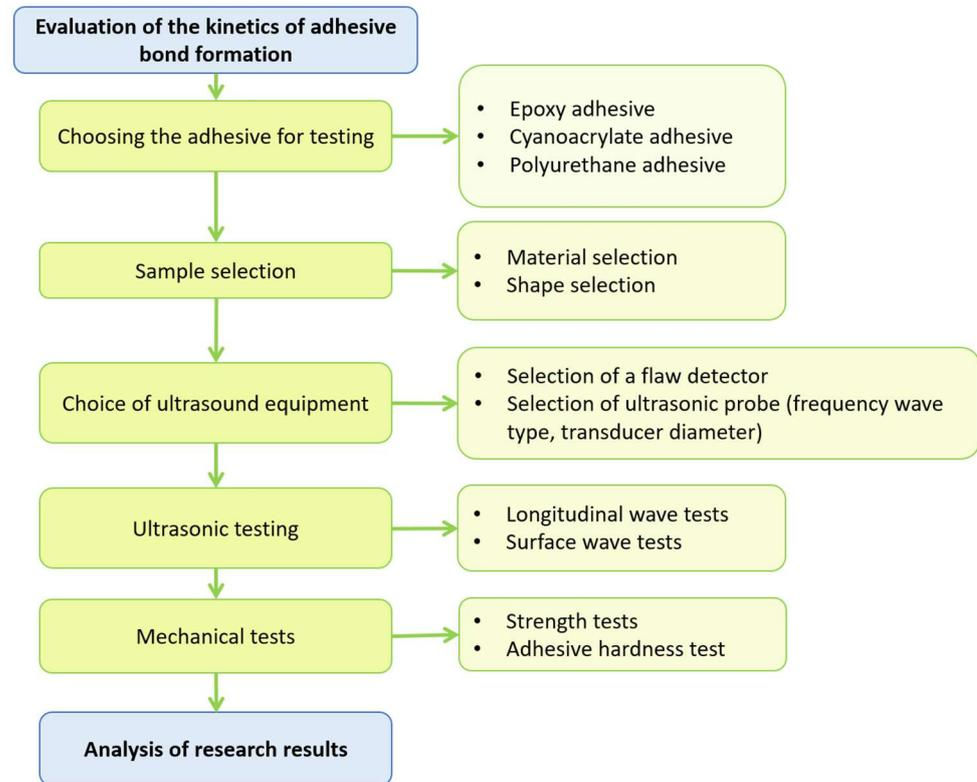
**Figure 1.** Research plan for the kinetics of adhesive bond formation.
