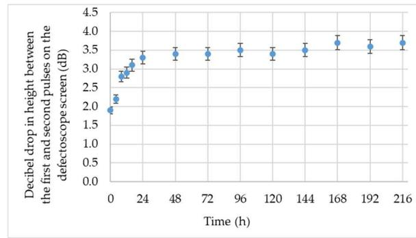
**Figure 12.** The change in decibel drop between the first and second pulses obtained on the screen of the ultrasonic defectoscope from the bond area for the ultrasonic test of bonded strips of steel sheet with epoxy adhesive.
