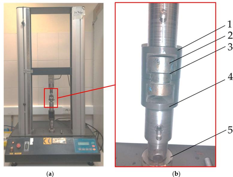
**Figure 9.** View of the testing machine (a) and the specimen clamped in the jaws of machine before rupture (b); 1—top clamping jaw, 2—glue sample, 3—glued joint, 4—bottom clamping jaw, and 5—bottom clamping to support machine.
