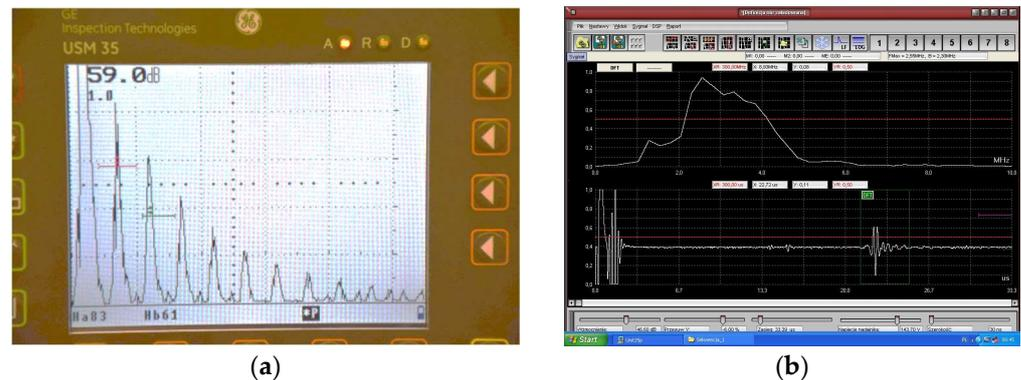
**Figure 7.** Examples of images of ultrasonic wave pulses recorded on digital defectoscopes screens: (a) in time domain, and (b) in time and frequency domain.
