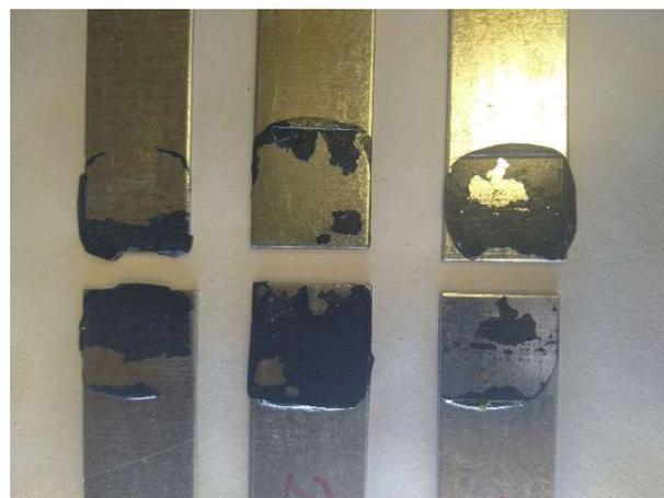
**Figure 17.** A view of torn steel strip bonds, mostly adhesive in nature.
