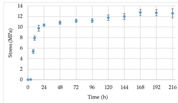
**Figure 15.** The distribution in time of the shear stresses for connected sheet metal strips.
