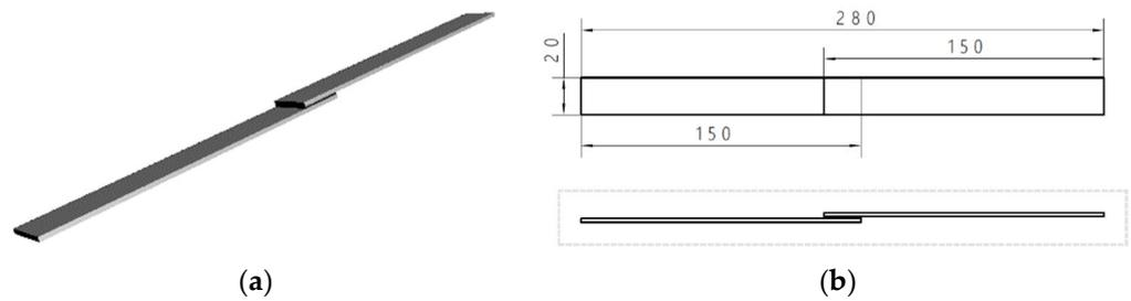
**Figure 4.** Sample used for testing—connected sheet strips for monitoring by ultrasonic longitudinal wave: (a) a view, and (b) dimensions—in millimeters.
