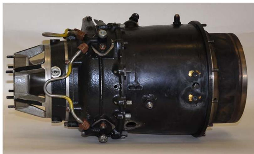
**Figure 2.** MPM-20 jet engine.
