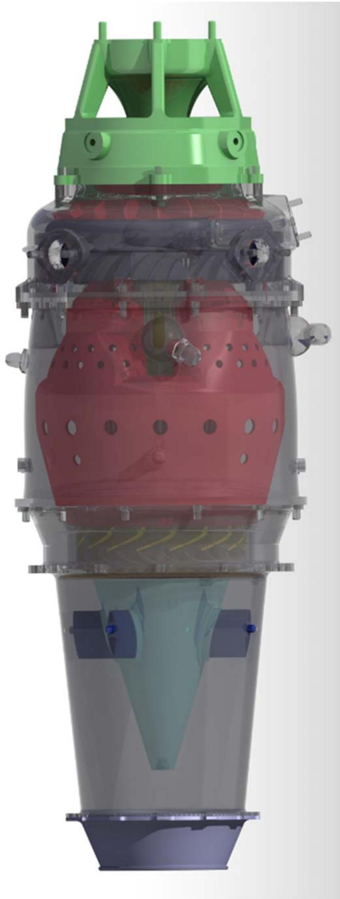
**Figure A2.** Visualization of the assembled MPM-20 jet engine.
