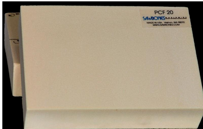
**Figure 1.** Image of the  $13 \times 20 \times 4$  cm polyurethane foam blocks used.
